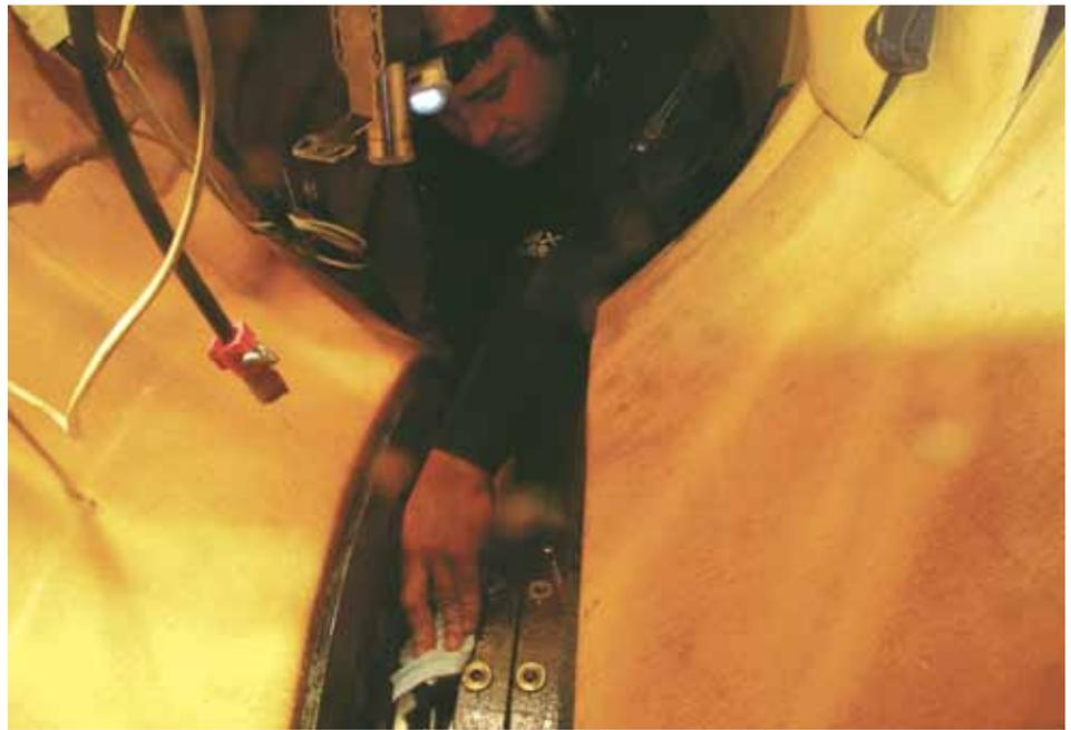
*The Hydrex 'mobdock' system enables sterntube seals to be replaced without drydocking*
