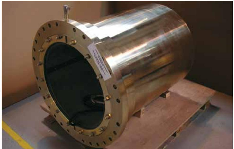
*An Orkot TXMM Mainshaft Bearing is made from machinable composite material*
