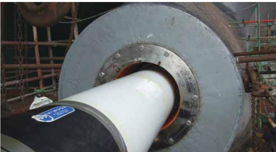
Under installation at Sembawang Shipyard, Singapore, this Compac bearing will provide zero sterntube oil leakage on a 141,000 dwt tanker
