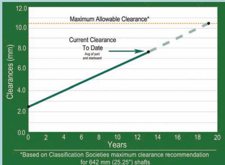
**Thordon compac seawater lubricated propeller shaft bearing clearances (for *Grand Princess*)**
