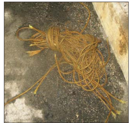
The remains of the rope that cause the oil leak.
