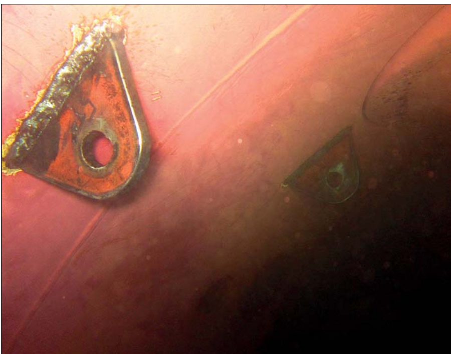
Pad eyes were installed in the thruster tunnel to secure the unit during removal.
