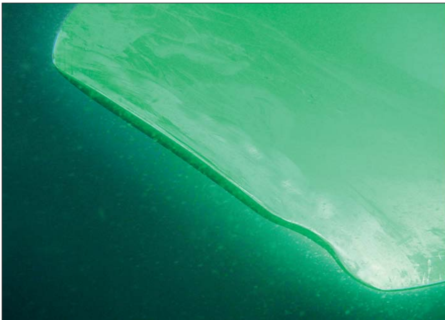
Cropped and polished blade of 225-meter bulk carrier.
