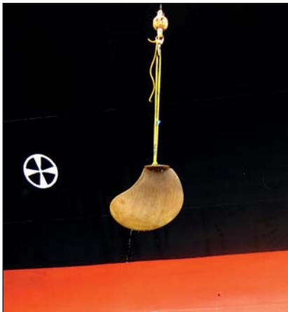
One of the bow thruster blades being brought to the surface.
