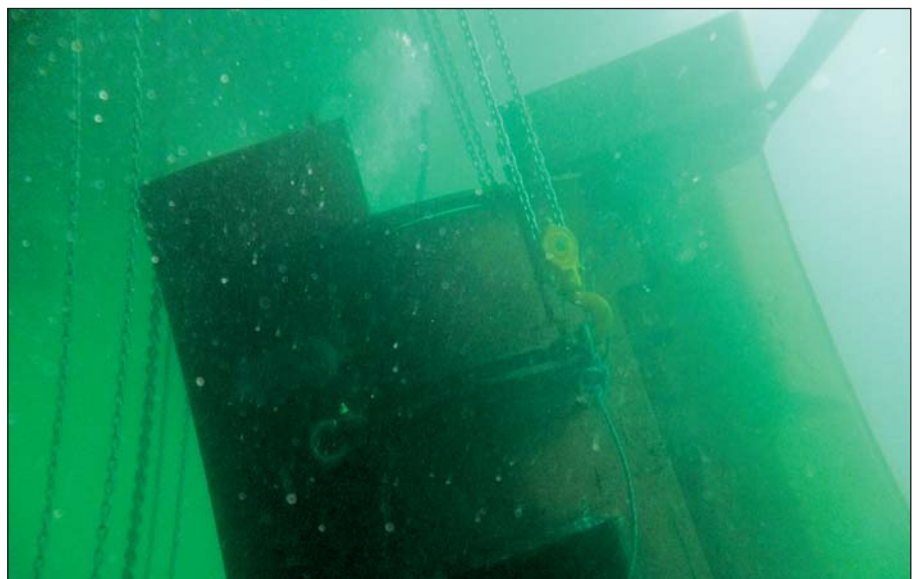
The rudder was secured with chain blocks and then slowly lowered.
