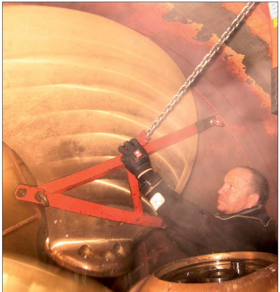
Lifting one of the old thruster blades inside the closed off thruster tunnel.
