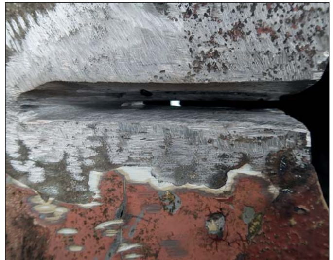
Ground out crack, ready to be filled.
