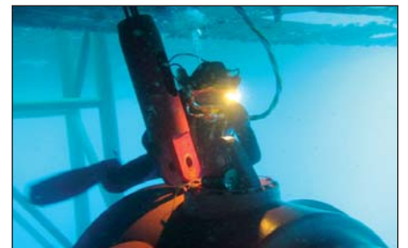
On-site repair on azimuth thruster in Gabon 10-12
