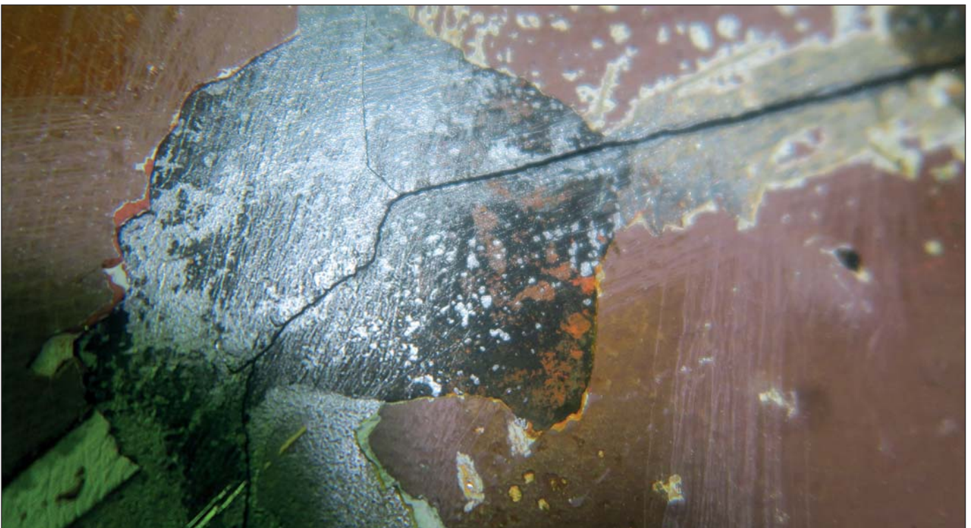
Branching crack on rudder of ro-ro ship.
