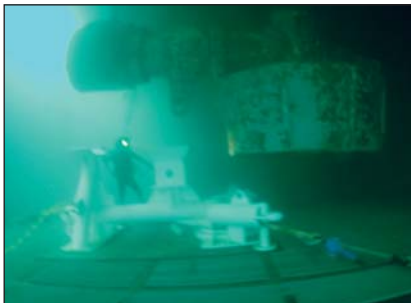
Lowering the thruster beneath the crane barge.
