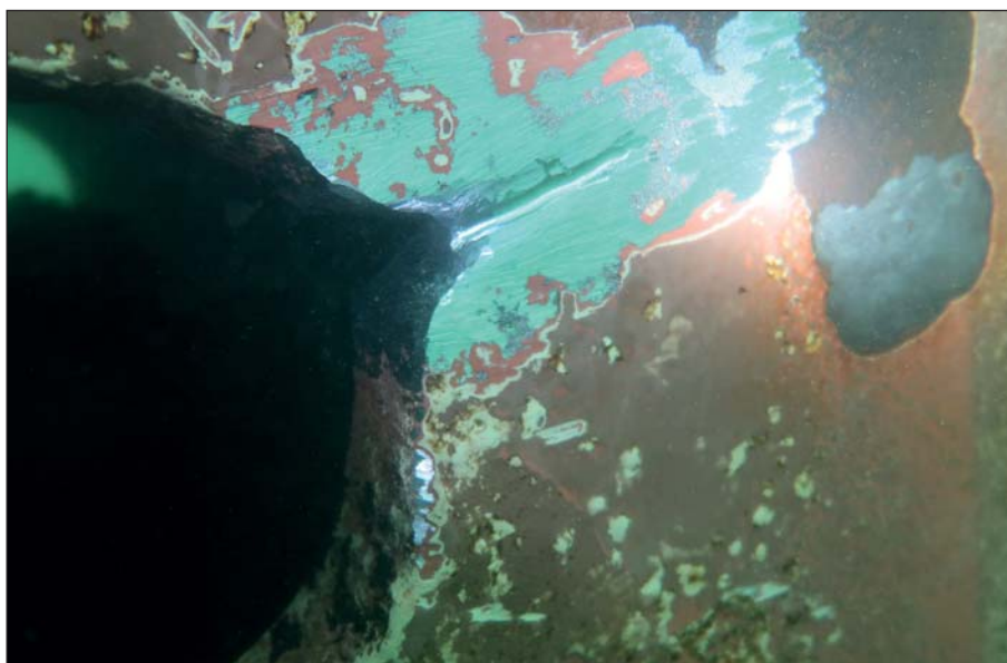
Ground out crack in upper rudder pintle corner of bulker in Dunkirk.
