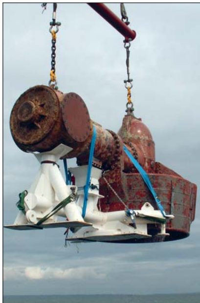
Transporting thruster out of water for repairs.
