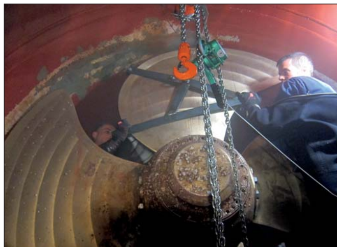
Positioning one of the new thruster blades.
