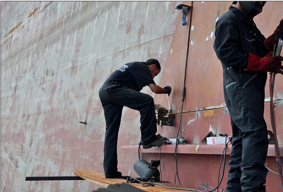
The top part of the doubler was then installed and connected to the bottom half.
