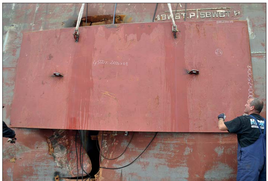
The lower part of the doubler plate being lowered from the deck.
