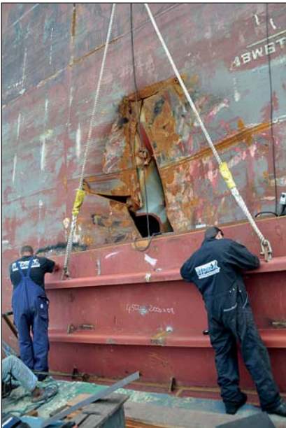
The doubler plate was given extra strength with horizontal stiffeners.
