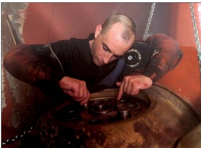
Hydrex diver/technician preparing the bow thruster unit for blade installation.
