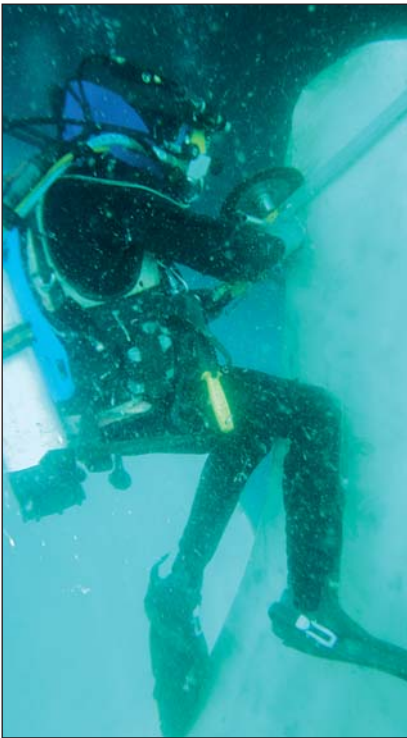
Hydrex diver cropping a propeller blade with the Hydrex cropping equipment.
