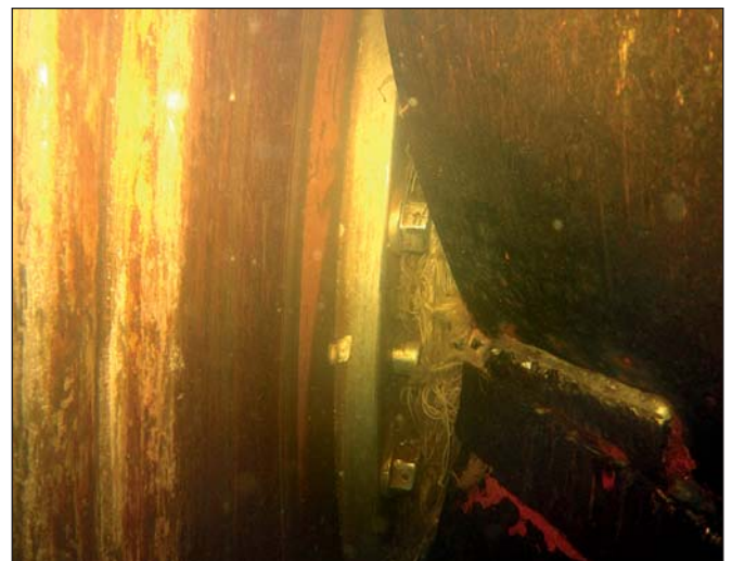
A rope in the stern tube seal assembly had caused damage to the rope guard.
