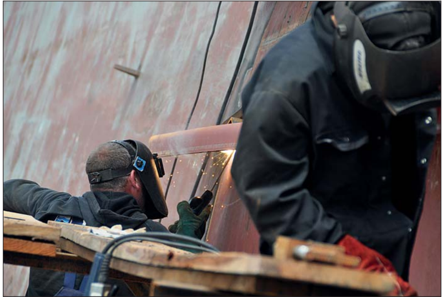
Hydrex certified welders working on the stiffeners.
