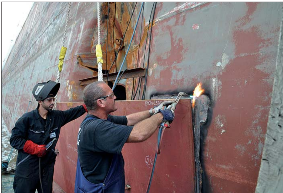
The bottom half of the doubler plate was fitted to the hull.
