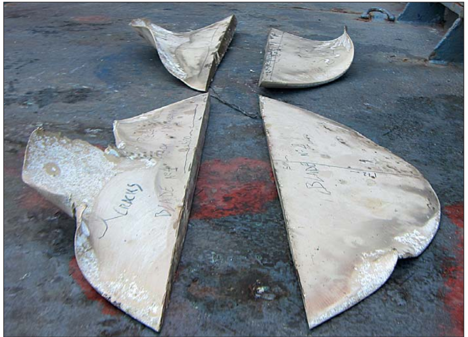
Four of the five propellers blades of the tanker needed to be cropped.
