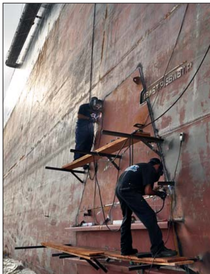
Hydrex certified welders securing doubler plate on bulker in Abidjan.
