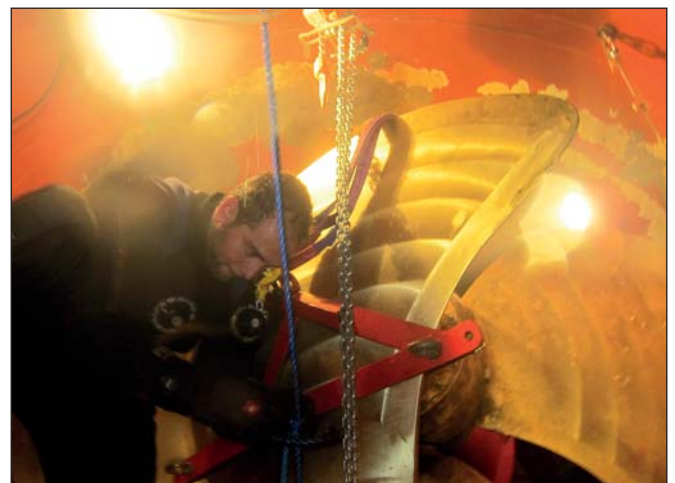
New bow thruster blade ready to be positioned in thruster tunnel.
