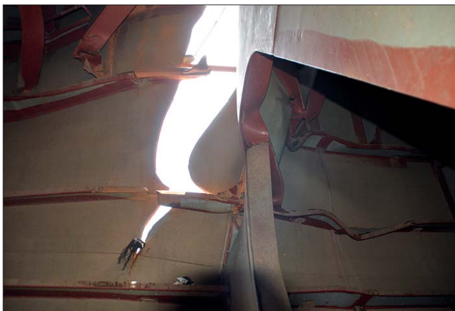
The damage was located in way of a ballast tank.
