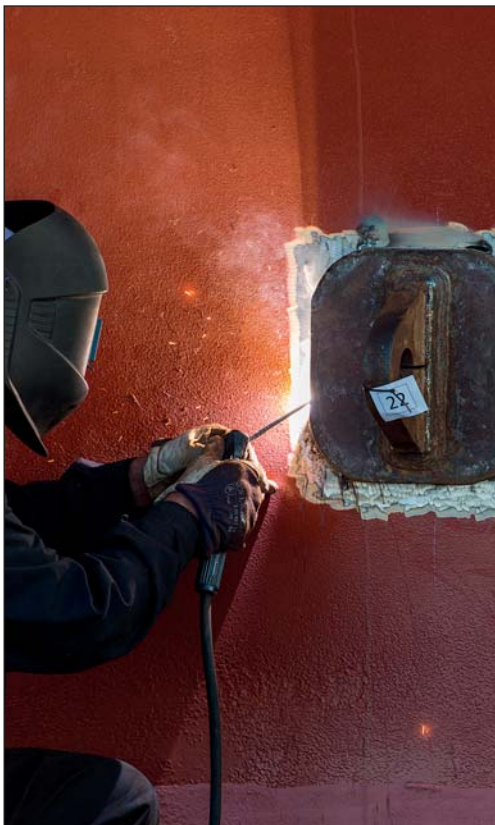
Preparation of the hull for the chains used to lower the unit.
