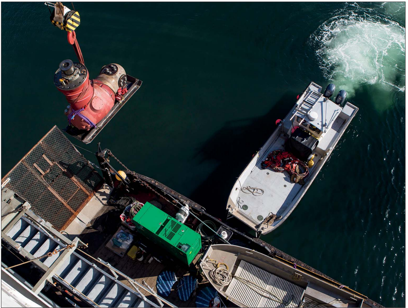
The bow thruster unit being lowered onto the workboat.
