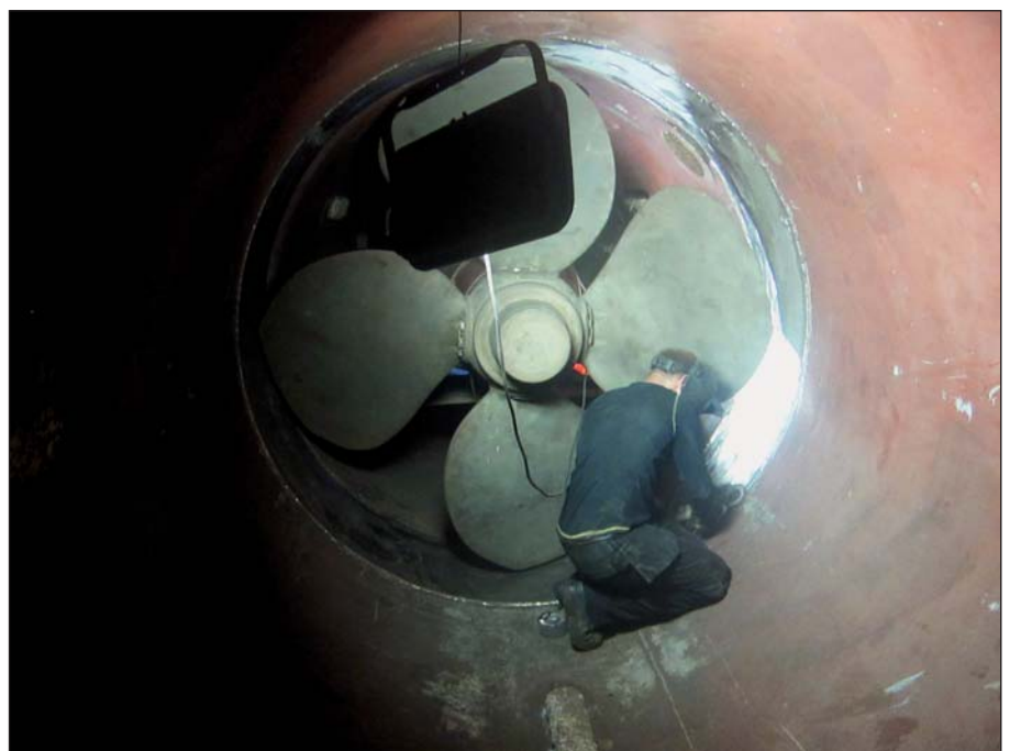
Hydrex technicians securing the new stainless steel belt.
