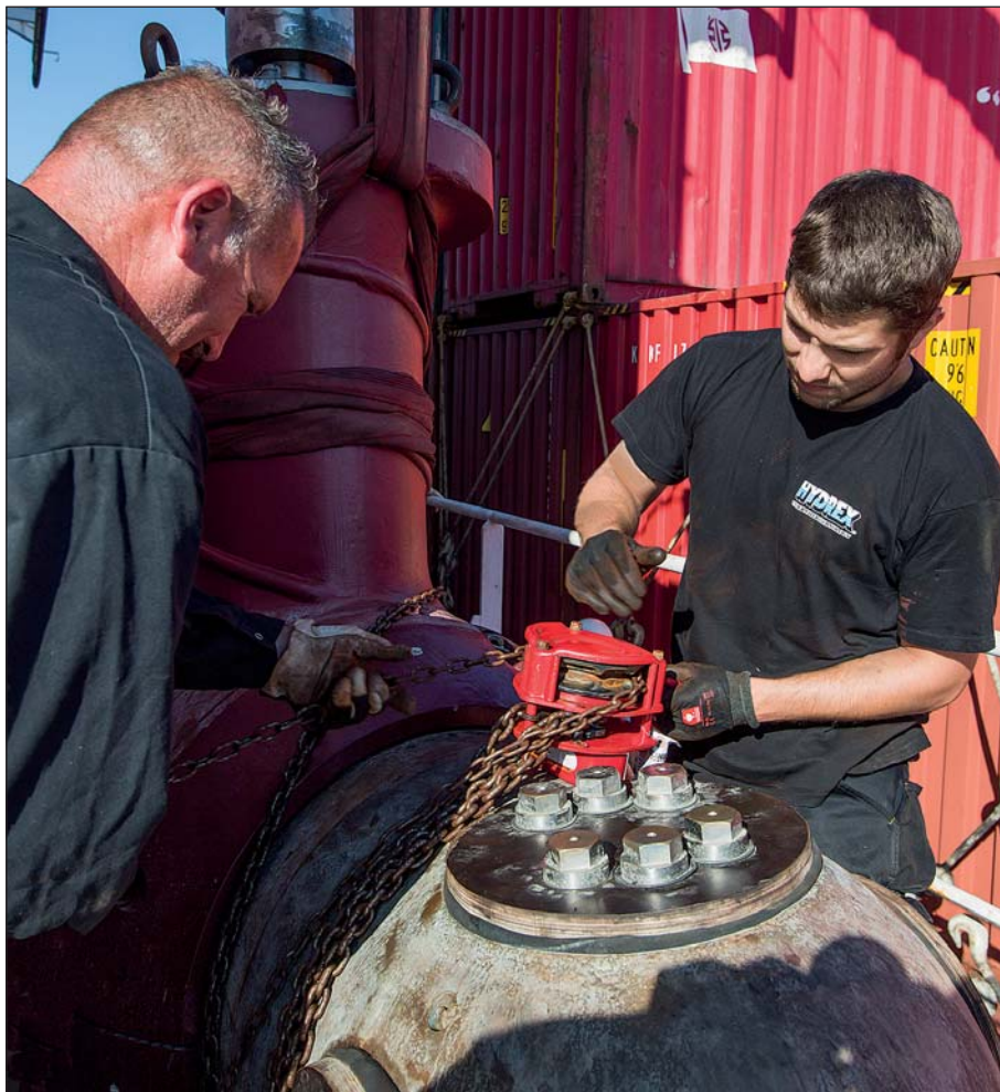
Hydrex diver/technicians preparing the bow thruster for reinstallation.
