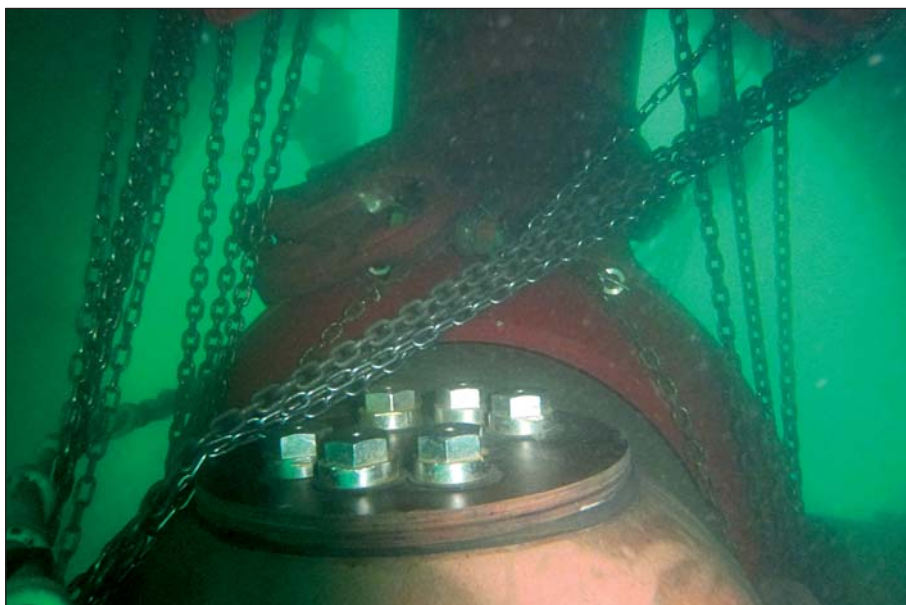
Bow thruster unit being positioned in the thruster tunnel.
