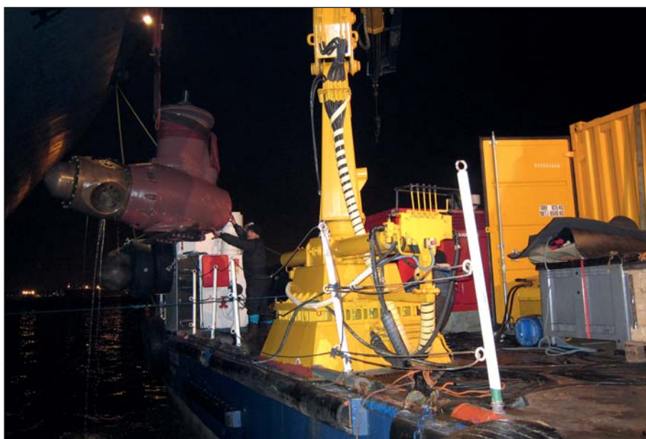
Bow thruster unit brought onboard the Hydrex workboat.
