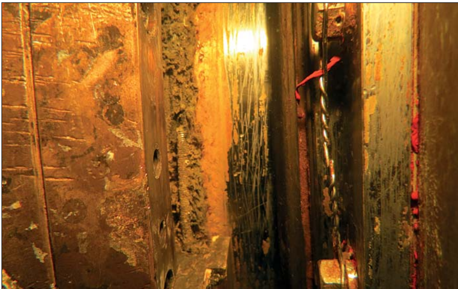
Heavily damaged running area of the stern tube seals.
