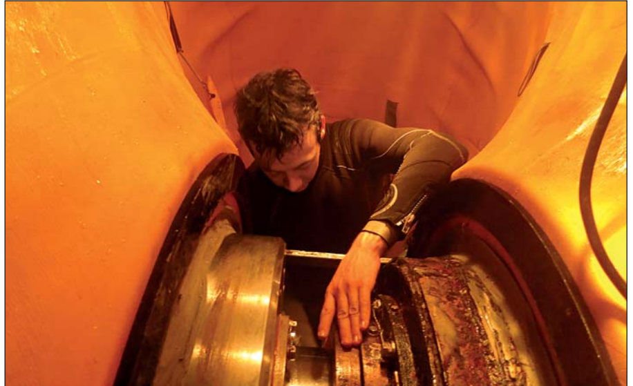
A dry environment is created inside the flexible mobdock.
