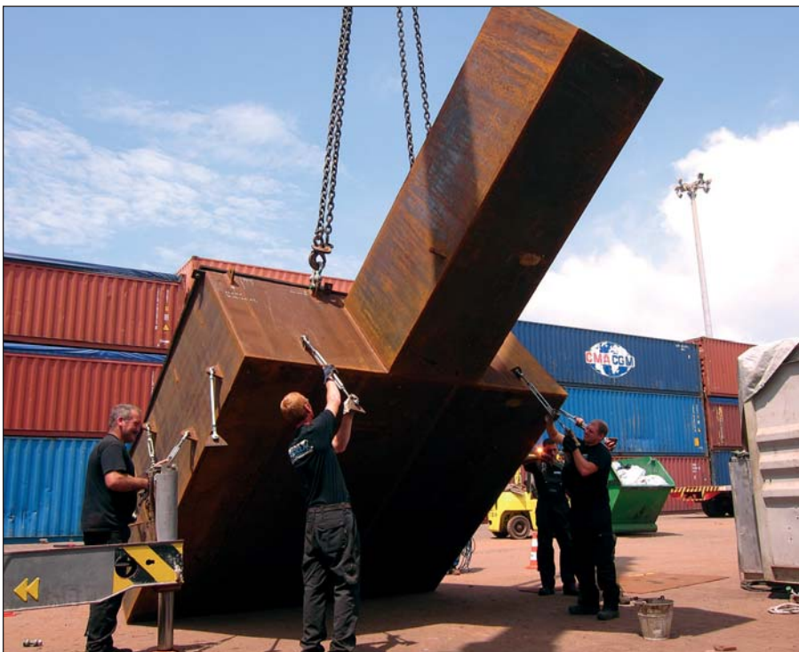
One of the cofferdams had an open top to give the Hydrex technicians access to the thruster tunnel.
