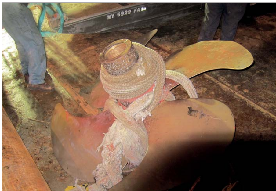
Propeller hub of the old unit, damaged by a mooring rope.
