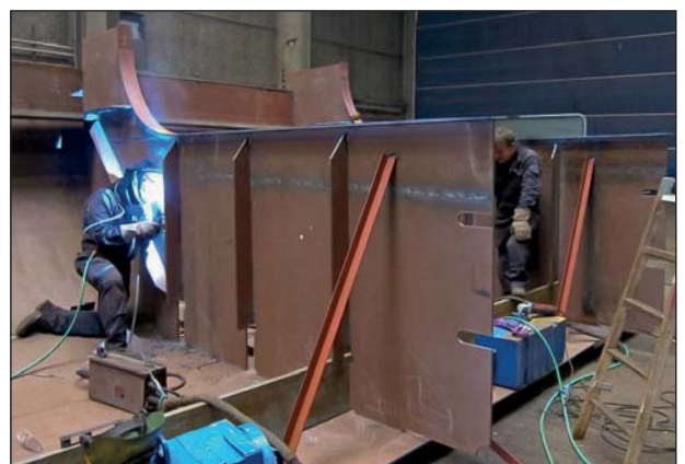
A custom solution was designed in cooperation with naval architects to perform the replacement of an entire section of an underwater hull.
