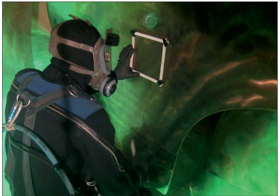
Hydrex designed a technique that allows work on a propeller to be carried out underwater, but in dry conditions.
