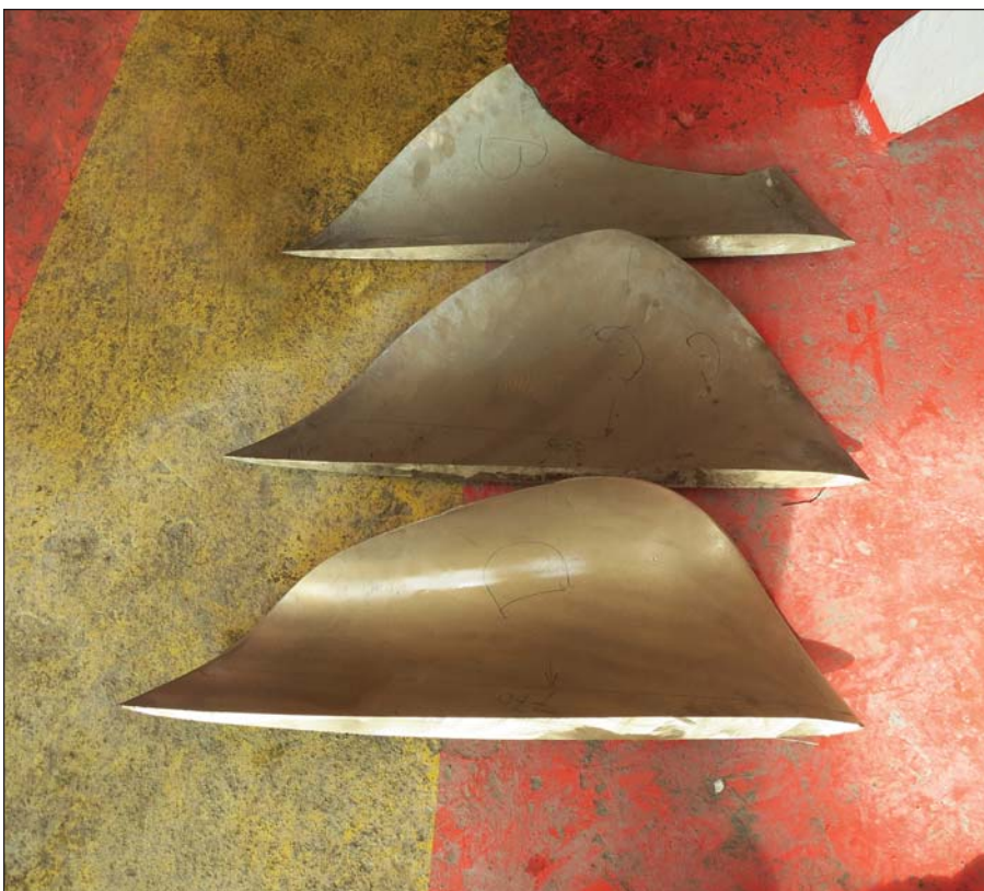
The bent blades were cropped one by one underwater.
