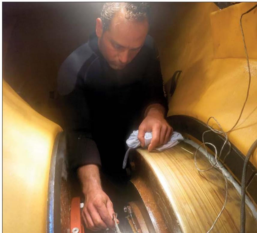
Using our flexible mobdock method to create a dry underwater environment, we have carried out stern tube seal repairs and replacements underwater for some years now in cooperation with top specialist suppliers.
