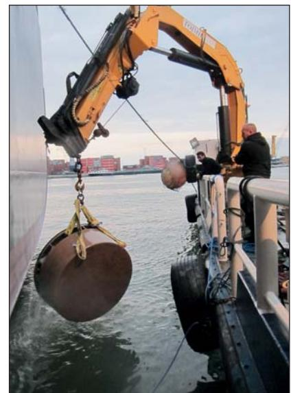
Old propeller cap being lifted out of the water with the hydraulic crane of the Hydrex workboat.
