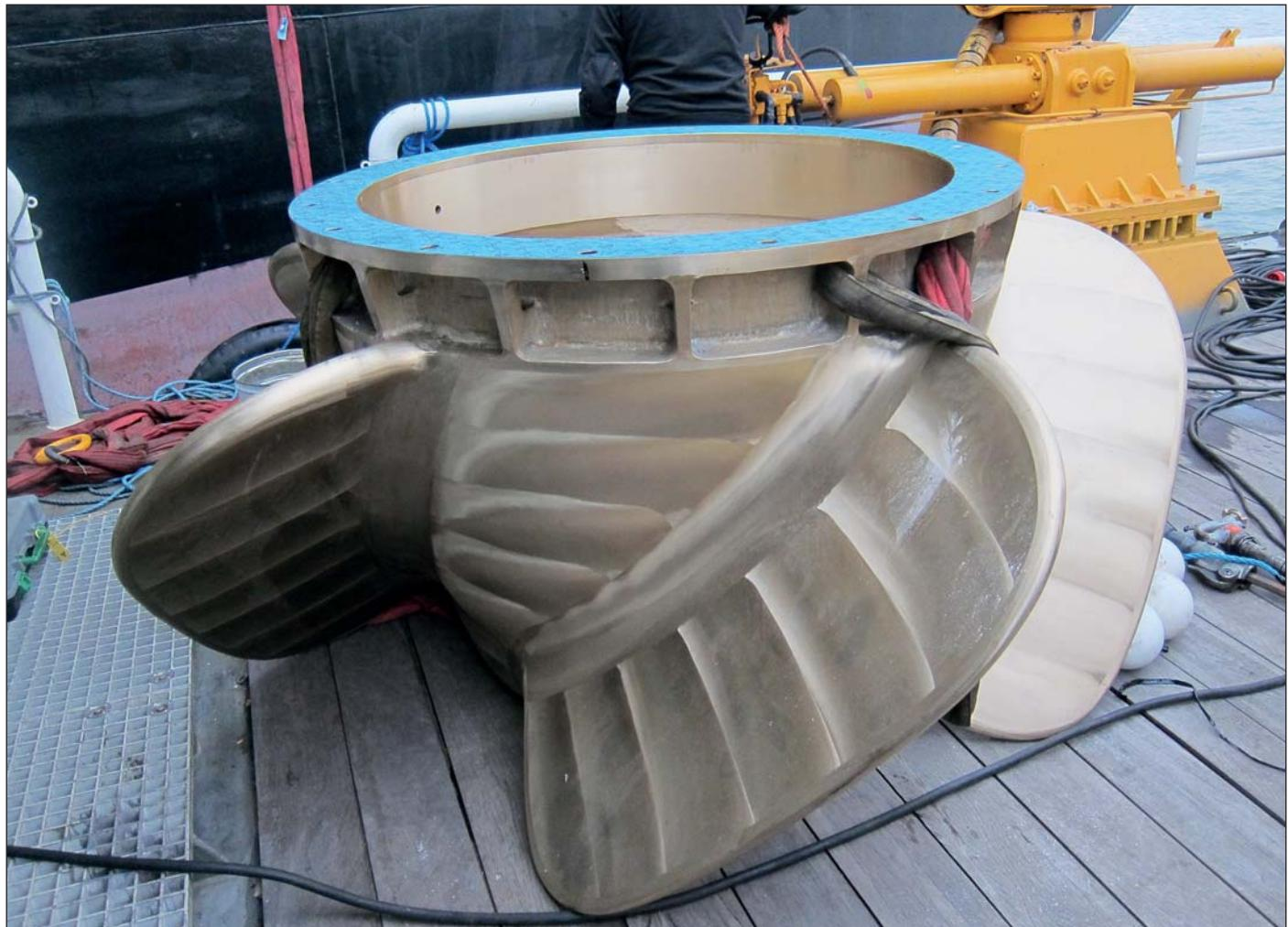
PBCF on Hydrex workboat, prior to installation.
