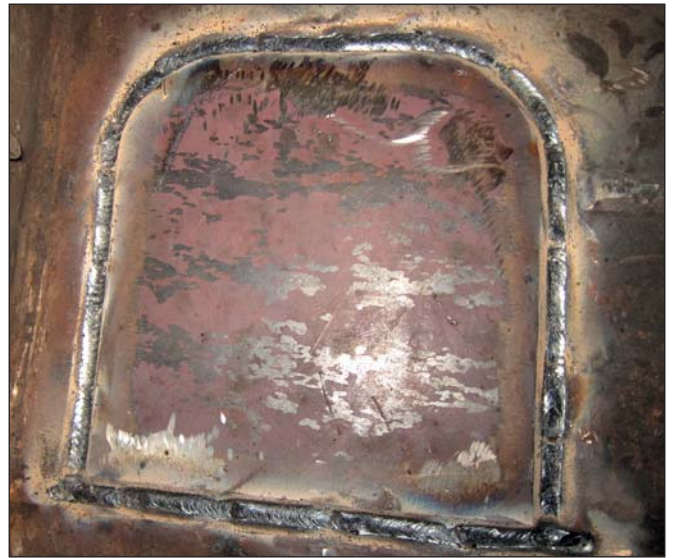
The new insert was secured with a full penetration weld.
