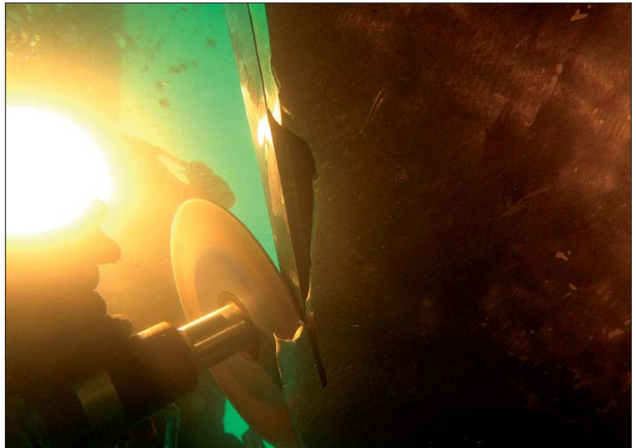
Propeller blade croppings are carried out with special cutting equipment developed by Hydrex.
