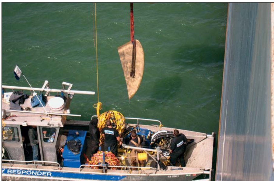
An identical part of the opposing blade was also cropped to restore the propeller's balance.
