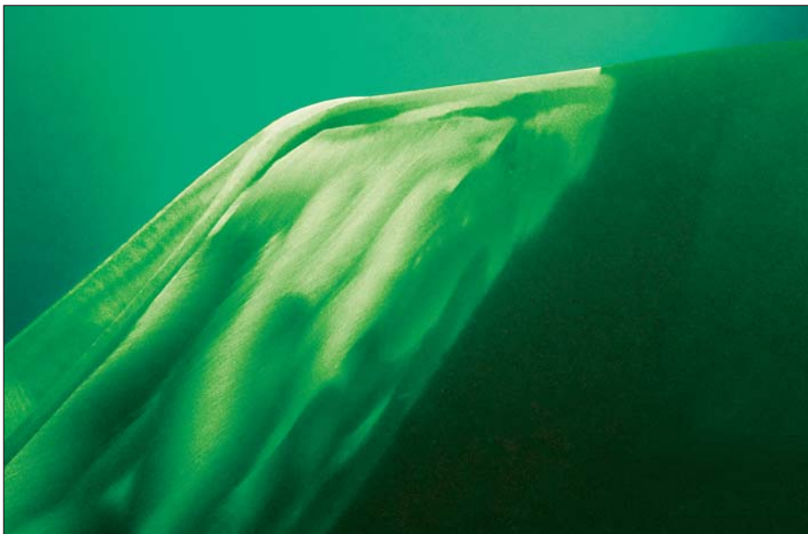
After cropping, the edges of the blade are smoothened to bring the propeller's efficiency back as close to its optimum condition as possible.
