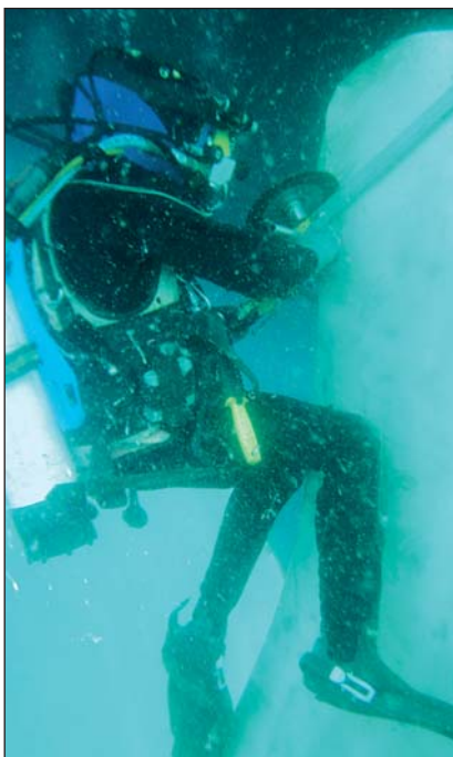
Hydrex diver cropping a propeller blade with the Hydrex cropping equipment.
