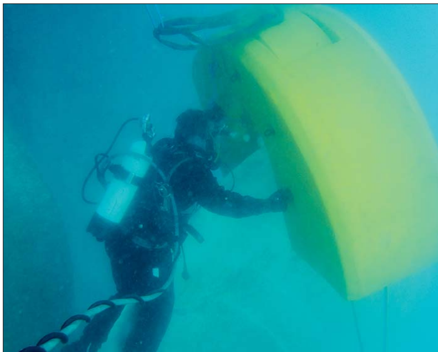
Hydrex diver positioning the cold straightening machine over a bent blade.
