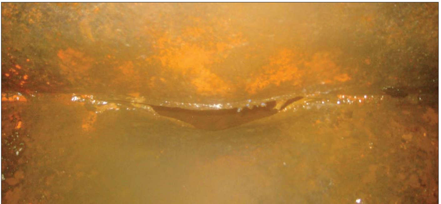
Crack in flat bottom plating of barge in Togo.
