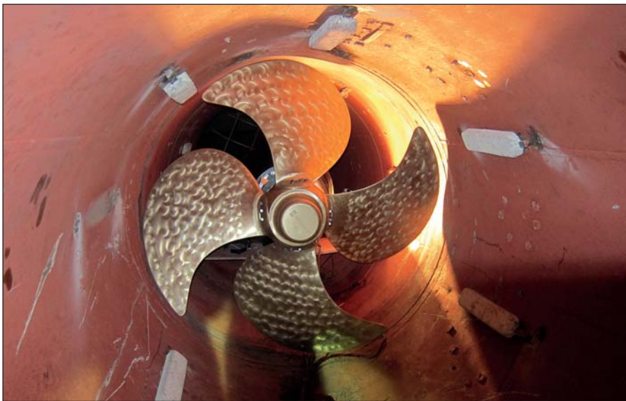
New bow thruster unit installed and secured.
