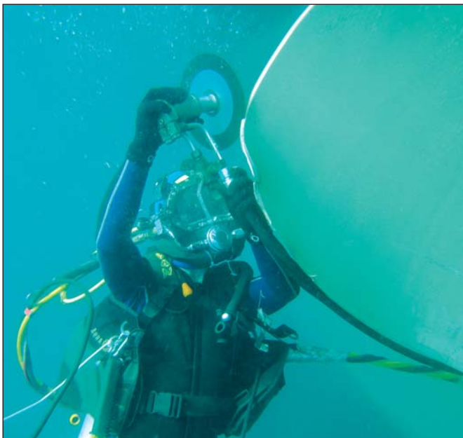
Hydrex diver/technician cropping the blade.
