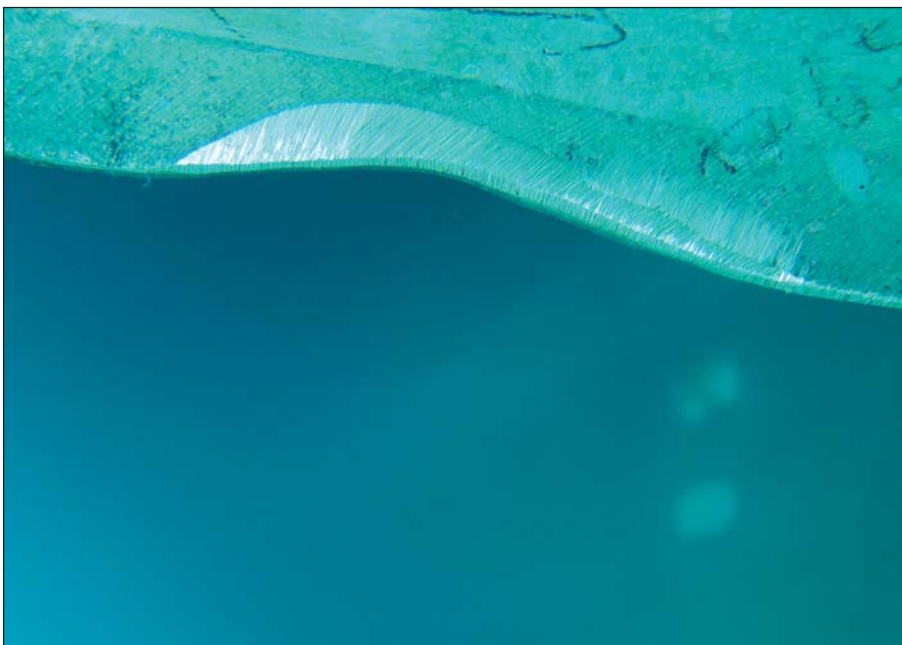
One of the repaired nicks along the trailing edge.
