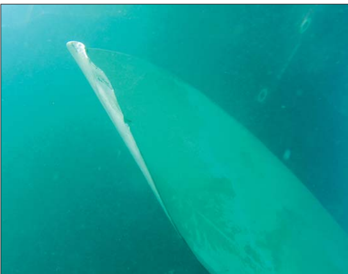
One of the blades was damaged by a buoy.
