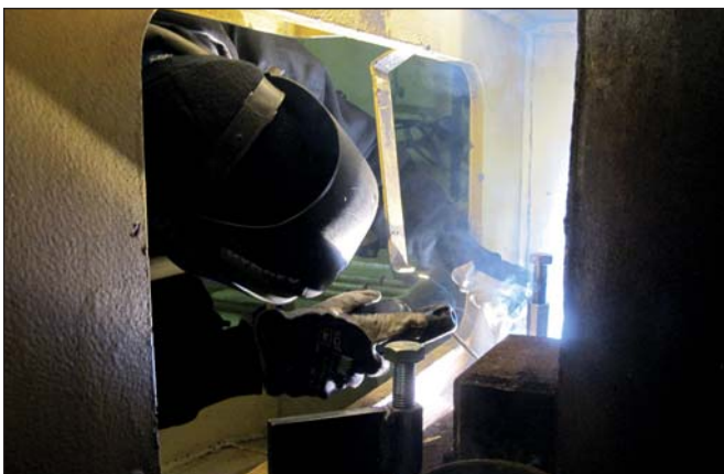
Hydrex diver working in the bow thruster room during thruster operation.
