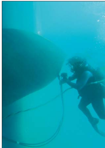
Cover: Hydrex diver grinding cropped propeller blade.
