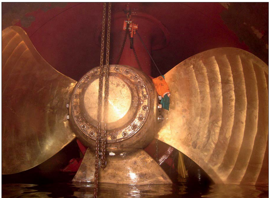
The bow thruster flexible mobdocks allow us to create a dry environment inside the thruster tunnel.
