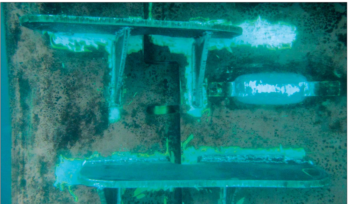
Girders were used to secure the flap to the rudder.
