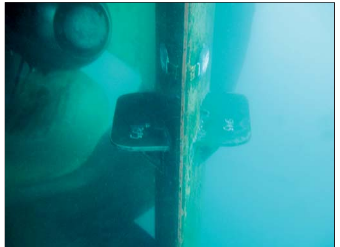
Three stiffeners were installed on each side of the rudder.
