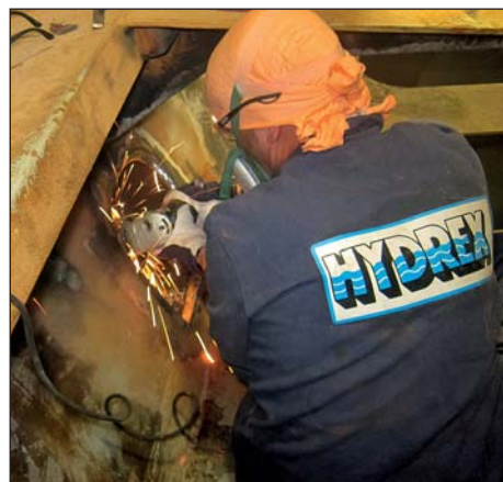
Preparing the edge of the opening for the new insert.
