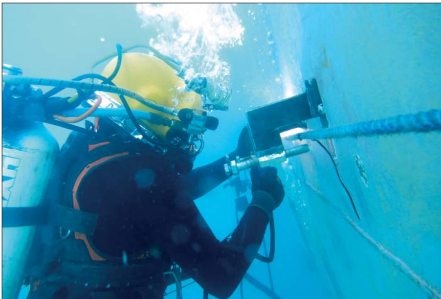
Preparing the hull for installation of the flexible mobdocks.
