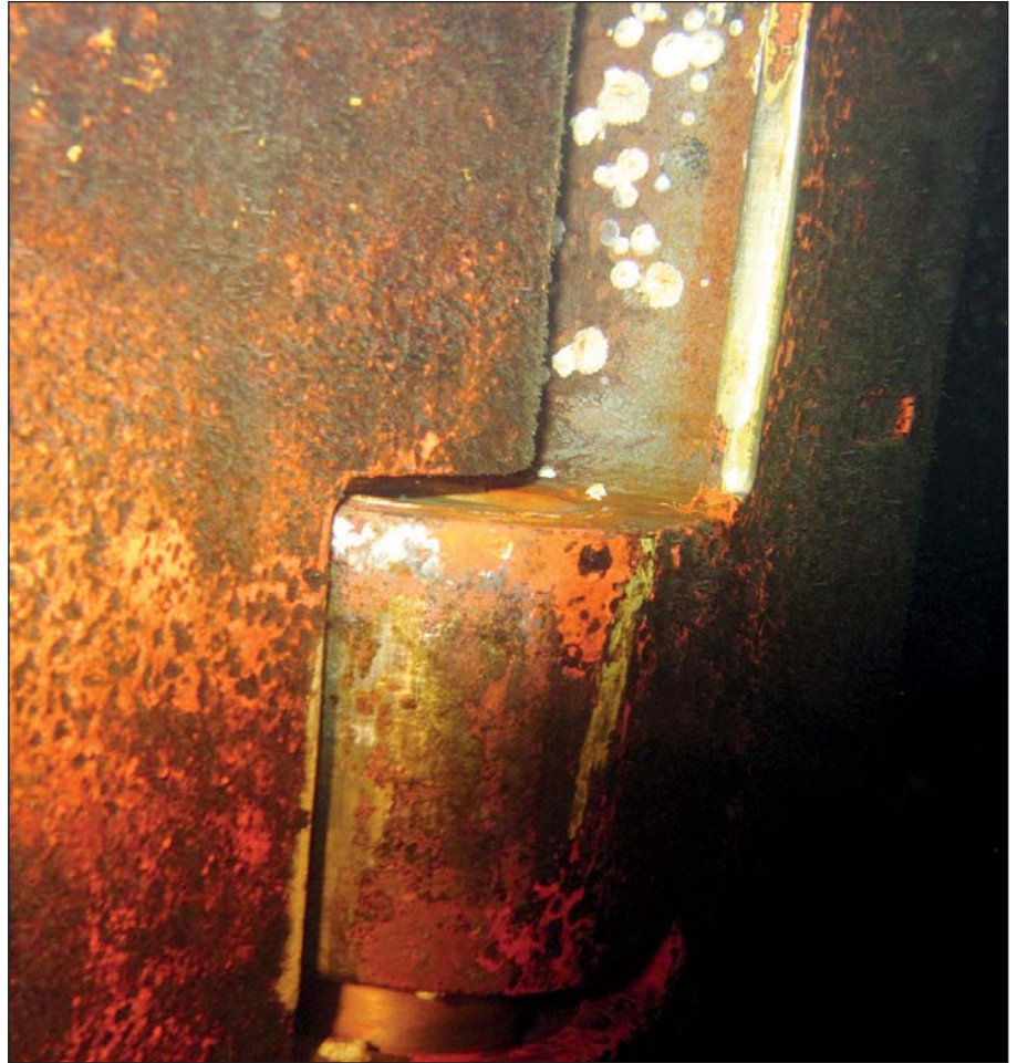
The top hinge of the rudder flap had come loose.
