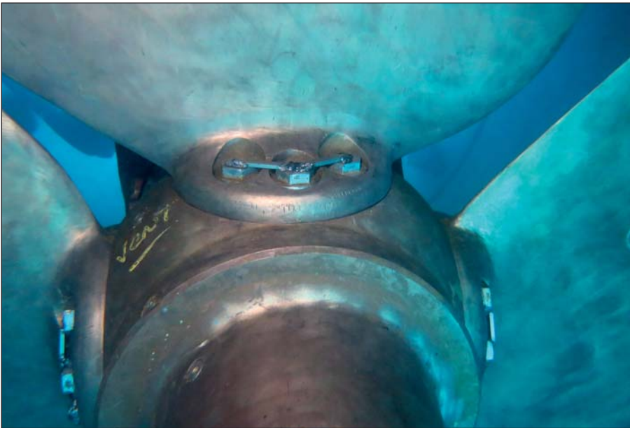
Reinstalled and secured thruster blades.
