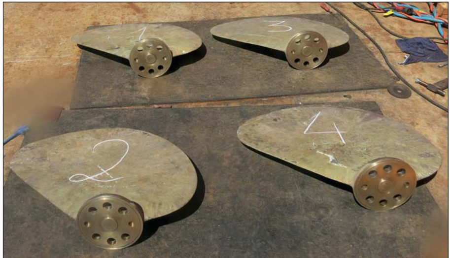
Bow thruster propeller blades after removal, prior to being refurbished.
