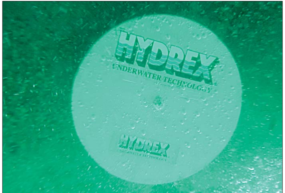
Temporary blank installed by Hydrex Spain.
