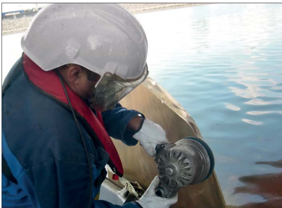
Buffing one of the cropped blades to achieve the best possible efficiency.
