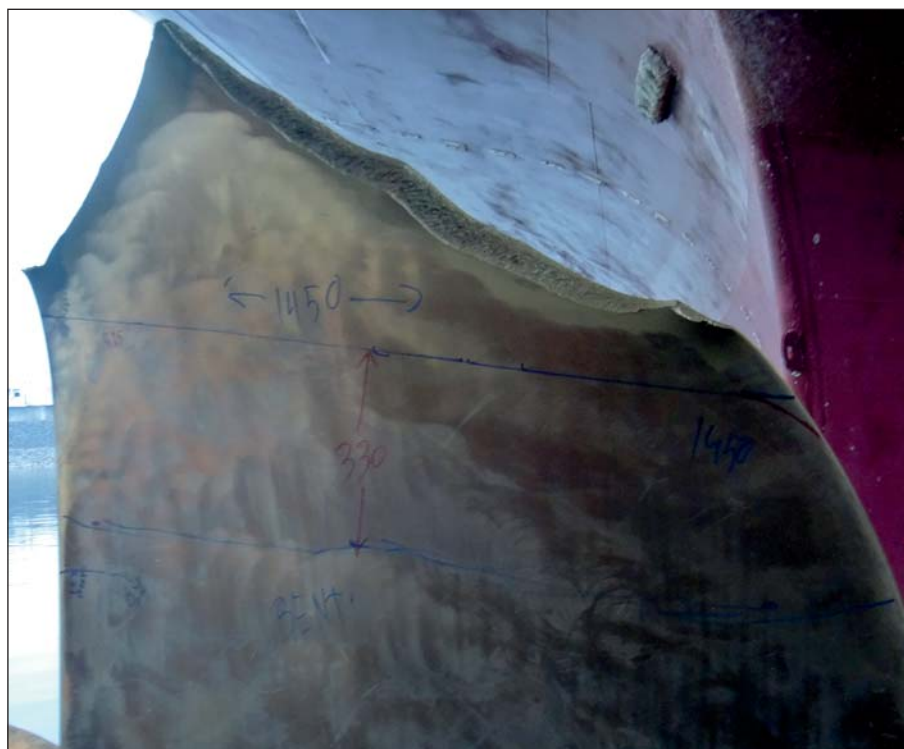
One of the propeller blades was missing parts of its tip.
