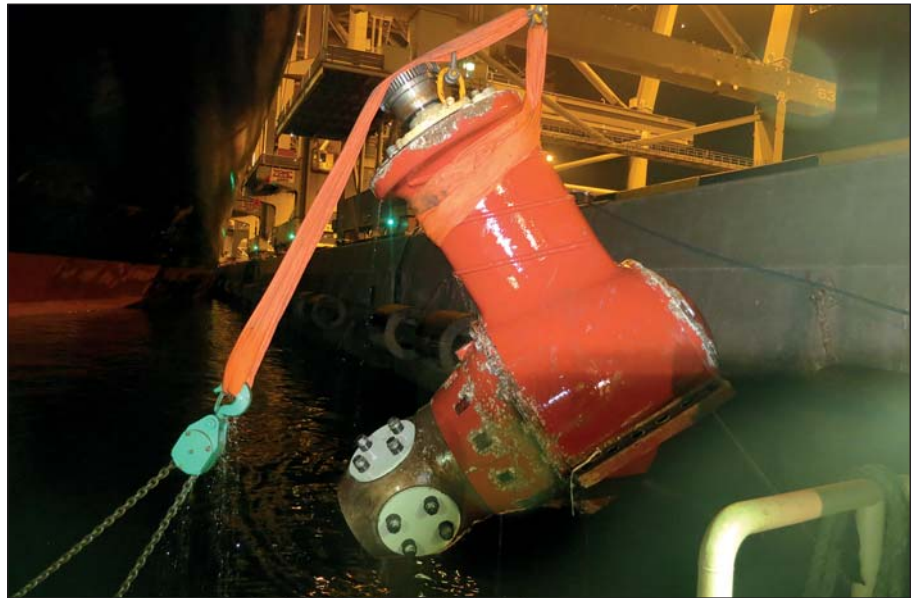
Bow thruster unit lifted out of the water.
