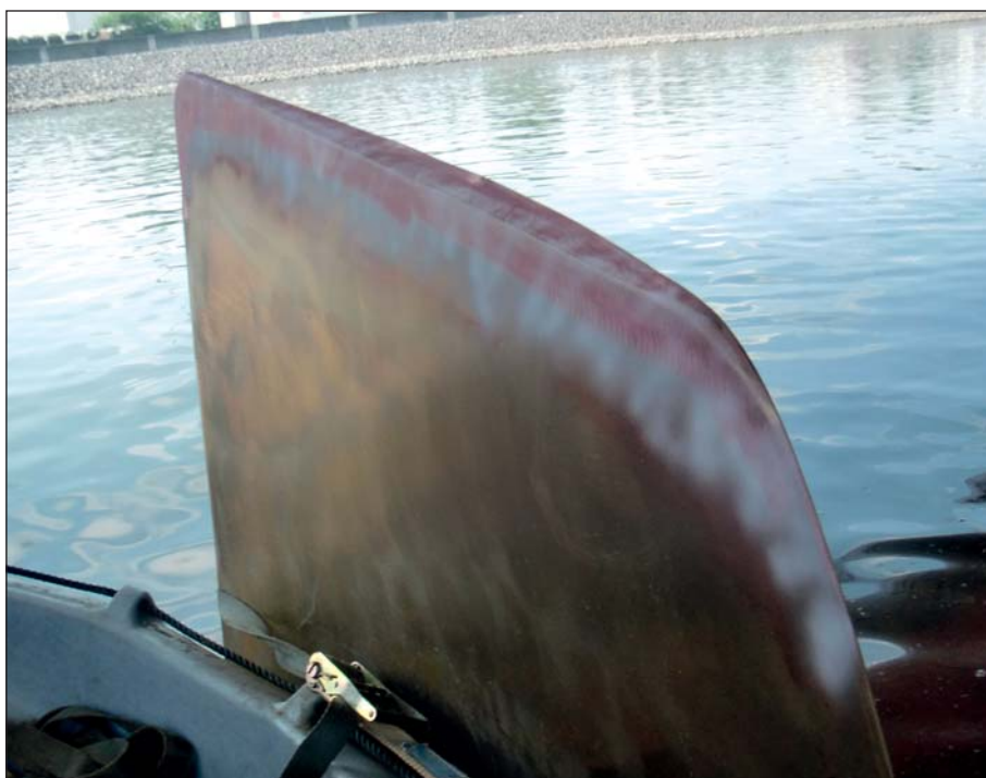
Testing one of the cropped blades for cracks.
