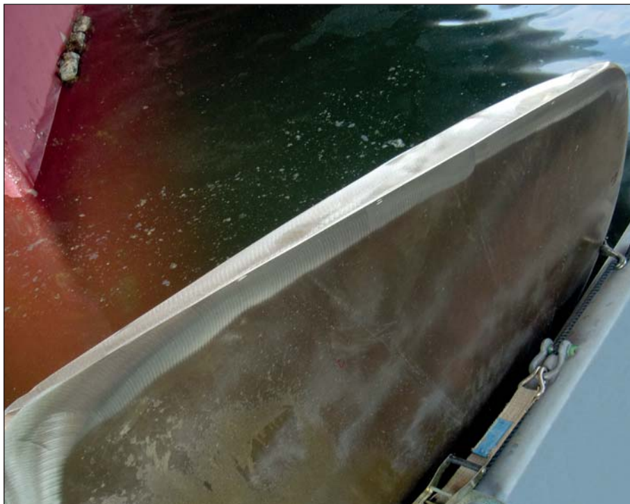
Cropped and buffed propeller blade.
