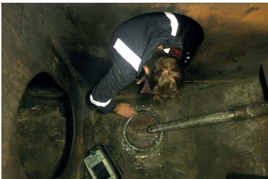
Independent ultrasonic tests were carried out on the weld seams.
