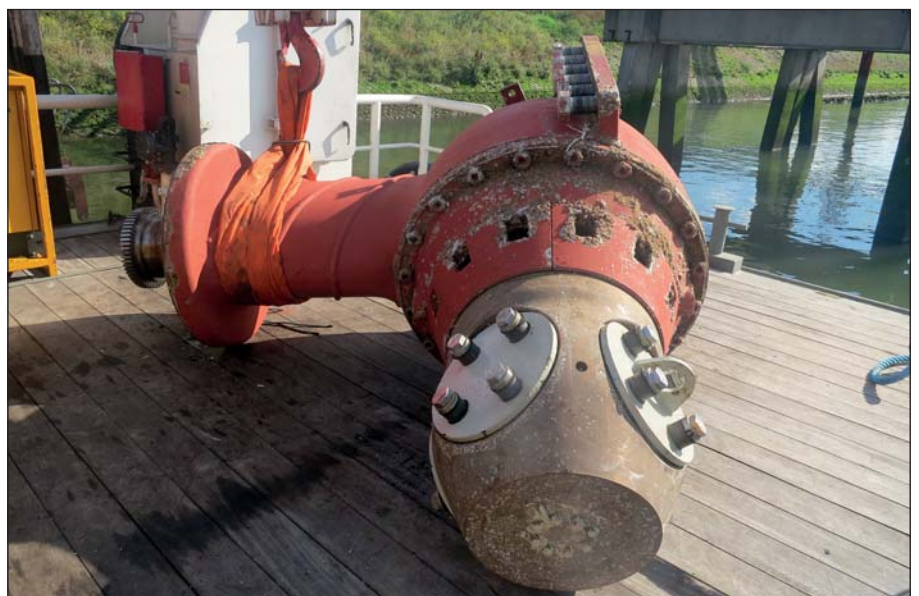
Thruster unit on Hydrex workboat.
