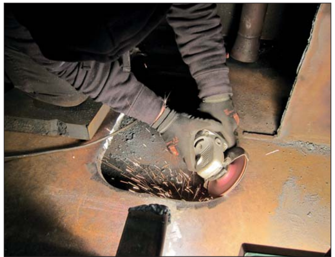
Preparing the edge of the hull plating to have a perfect fit for the new plate.
