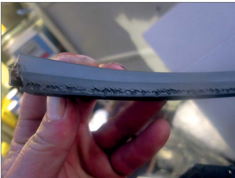
One of the damaged seals that caused the oil leak.
