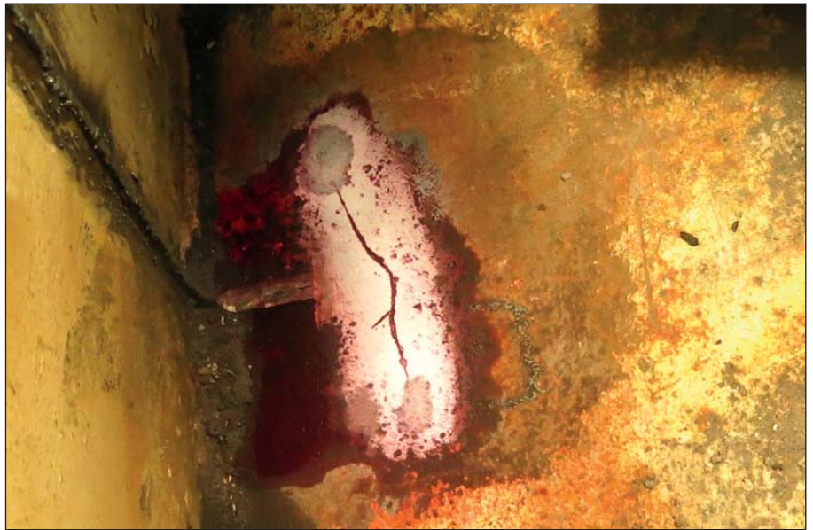
Crack in the bottom plating of tanker in Antwerp.
