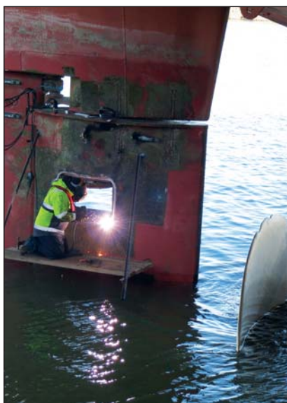
Cover: Preparing the rudder for installation of the new cover plates.
