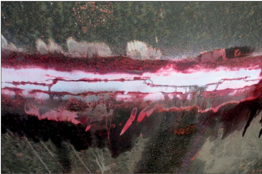
A dye check revealed the extend of the cracks.
