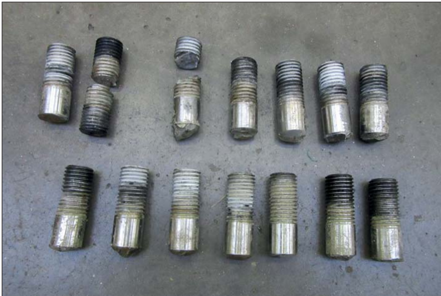
What was left of the bolts had to be removed carefully to protect the screw thread in the mounting flange.
