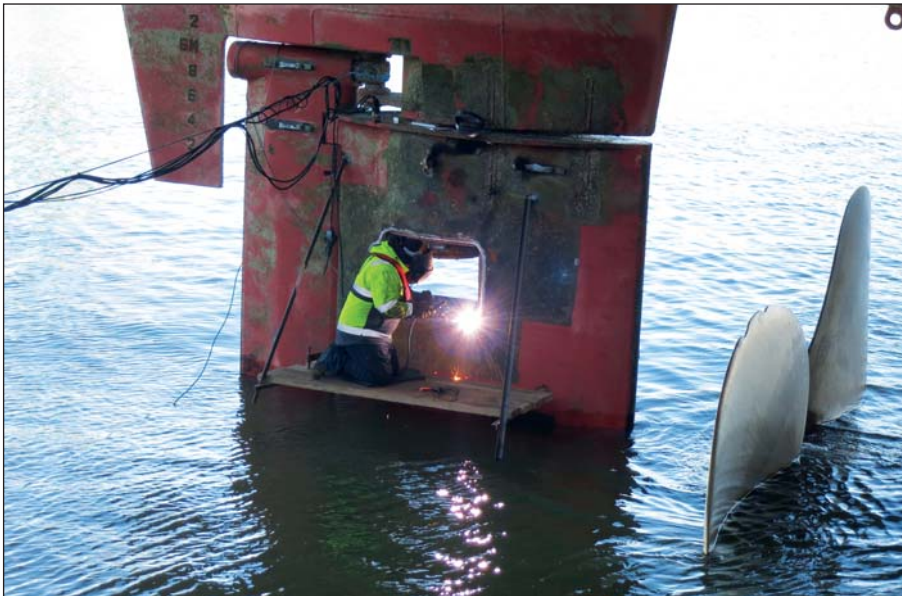
Preparing the rudder for installation of the new cover plates.
