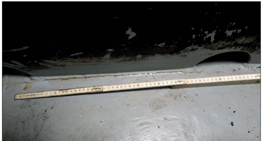
Crack in grey water tank seen from the outside ... and the inside.
