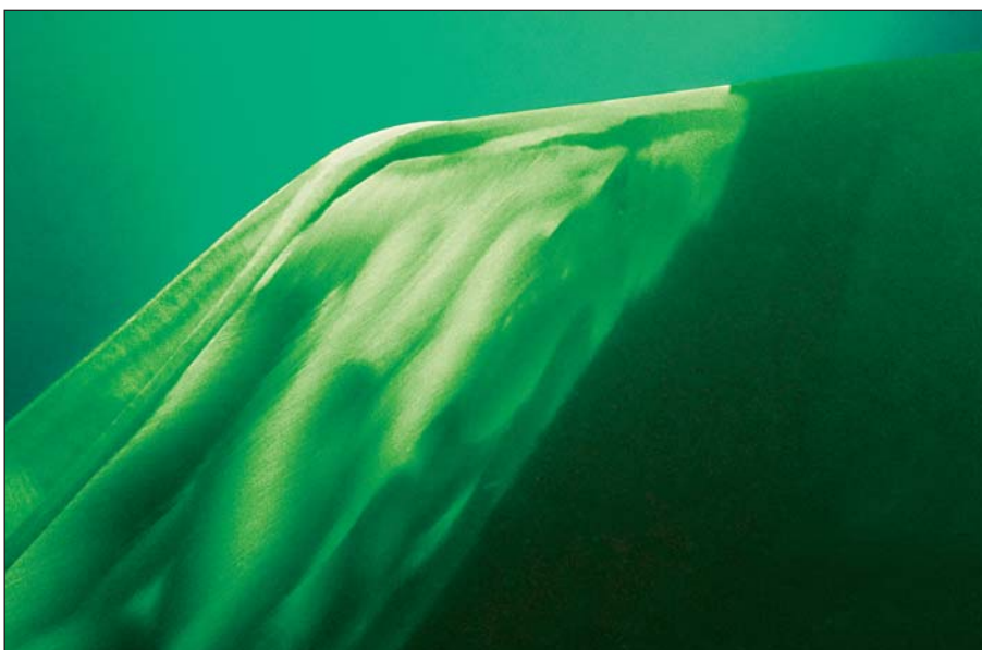
After cropping, the edges of the blade are smoothed to bring the propeller's efficiency back to its optimum condition.
