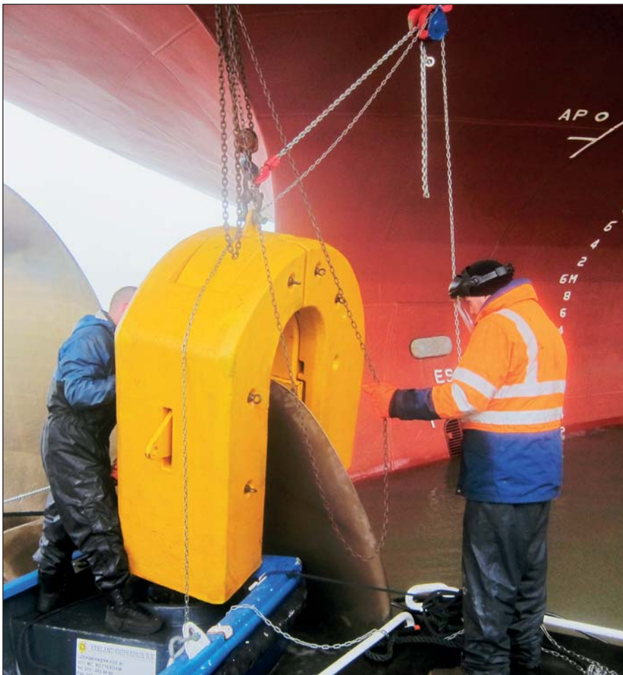
Hydrex cold straightening machine during operation above water.
