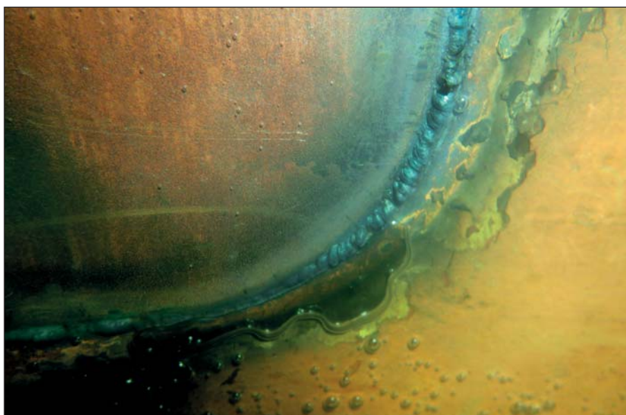
Full penetration weld as seen from the outside of the hull.
