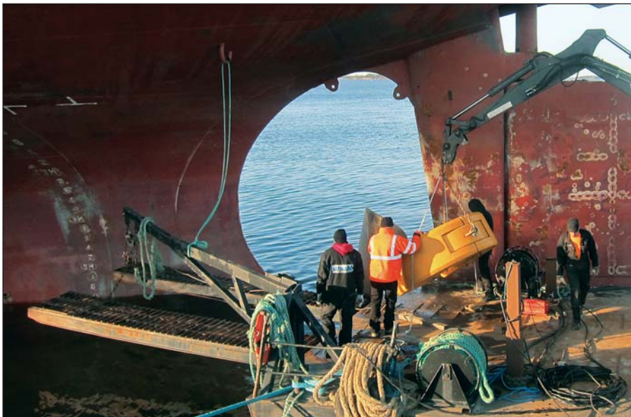
Diver/technicians positioning the latest version of the Hydrex cold straightening machine over a bent propeller blade.
