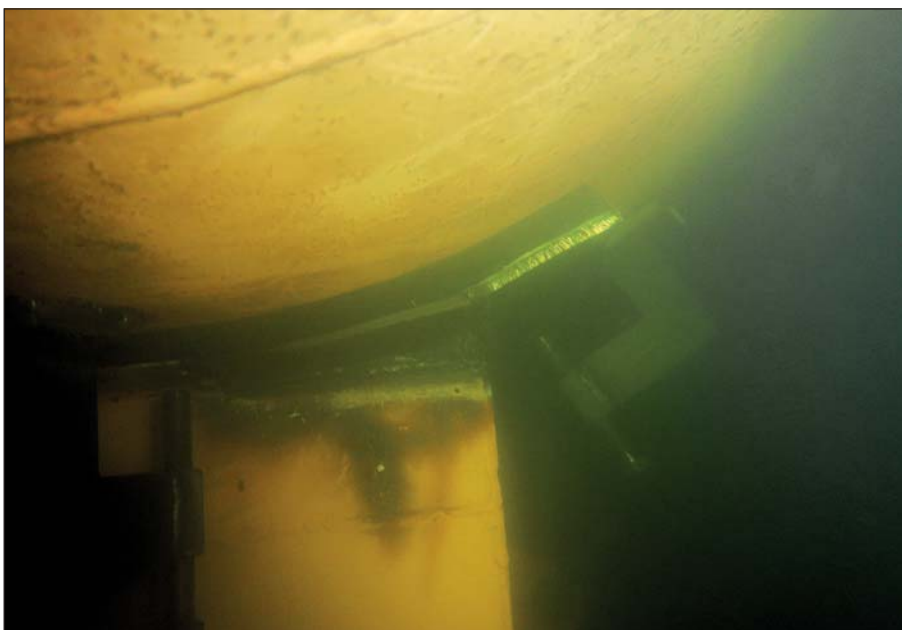
A special mobdock was constructed that would perfectly fit the shape of the hull.
