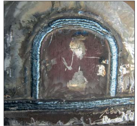
Full penetration weld.
