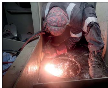
Installation of new echo sounder in a single day 4-6
