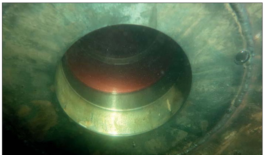
The new echo sounder flange seen from the outside.
