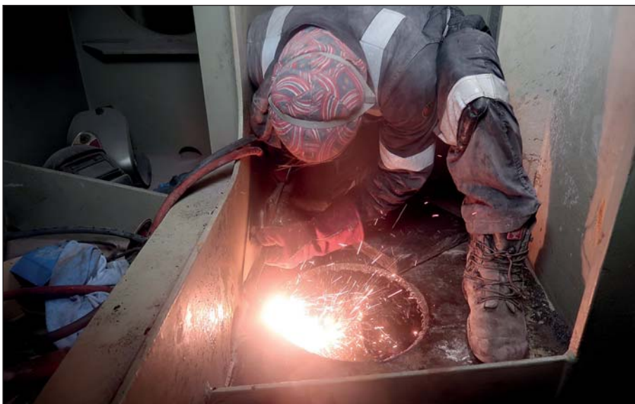
Removing the shell plating for installation of the new transducer system.
