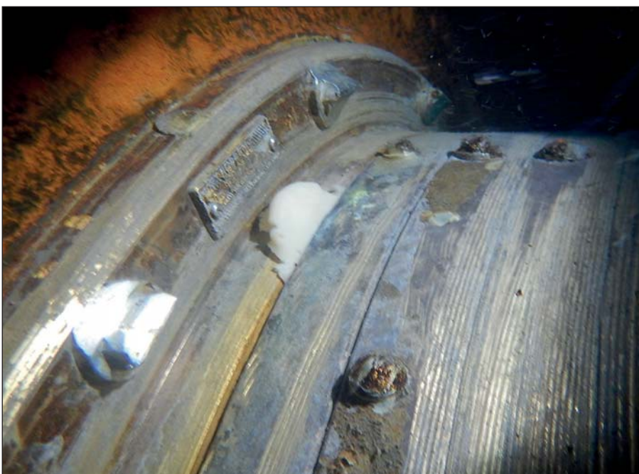
Oil leaking from the damaged seal housing.
