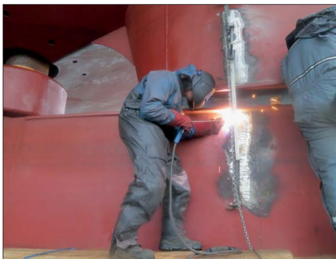
Hydrex certified welders securing the stiffeners.
