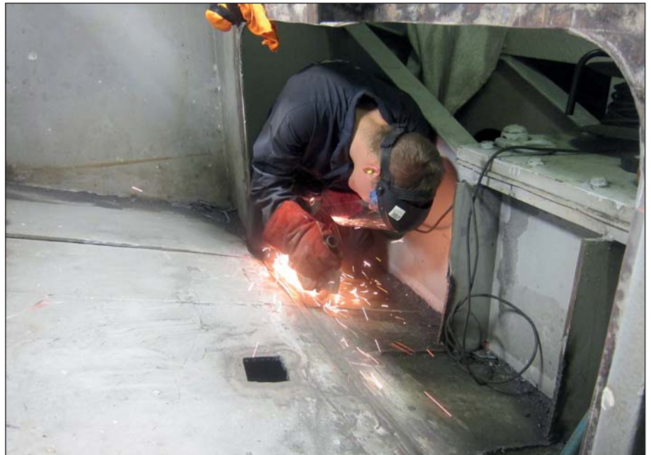
Hydrex diver/technician cutting away the damaged area during an insert repair.
