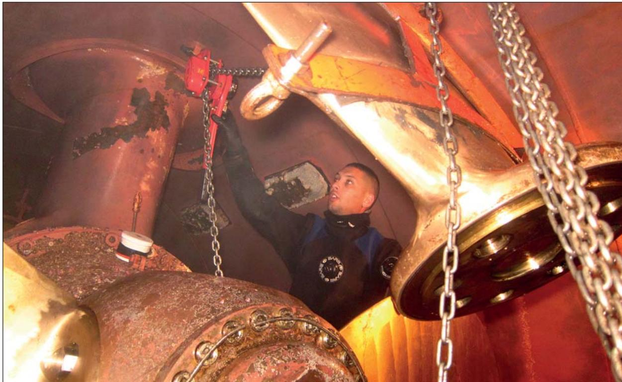
The Hydrex lightweight flexible mobdocks are designed to be easily transported around the world and are used to close off the thruster tunnel on both sides, allowing divers to perform repairs and other operations in a dry environment around the bow thruster unit.
