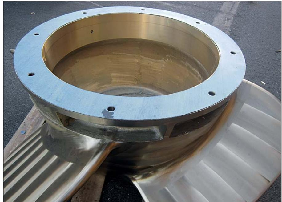
*Propeller cone fine ready for installation.*
