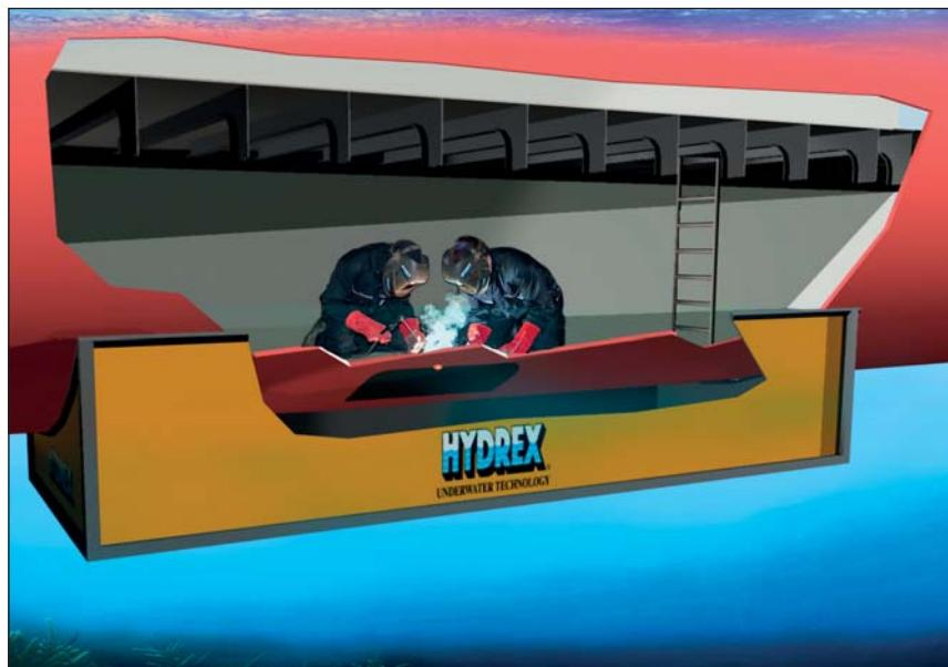
**H**ydrex on-site hull repair services include the renewal of both small and large areas of damaged hull plating. These repairs can be carried out above or below water, according to the circumstances, with tailor-made mobdock. Normal commercial activities can therefore continue without disruption. These operations follow the Hydrex procedure for welding cracks in the vessel's shell plating and they are approved by the major classification societies.
