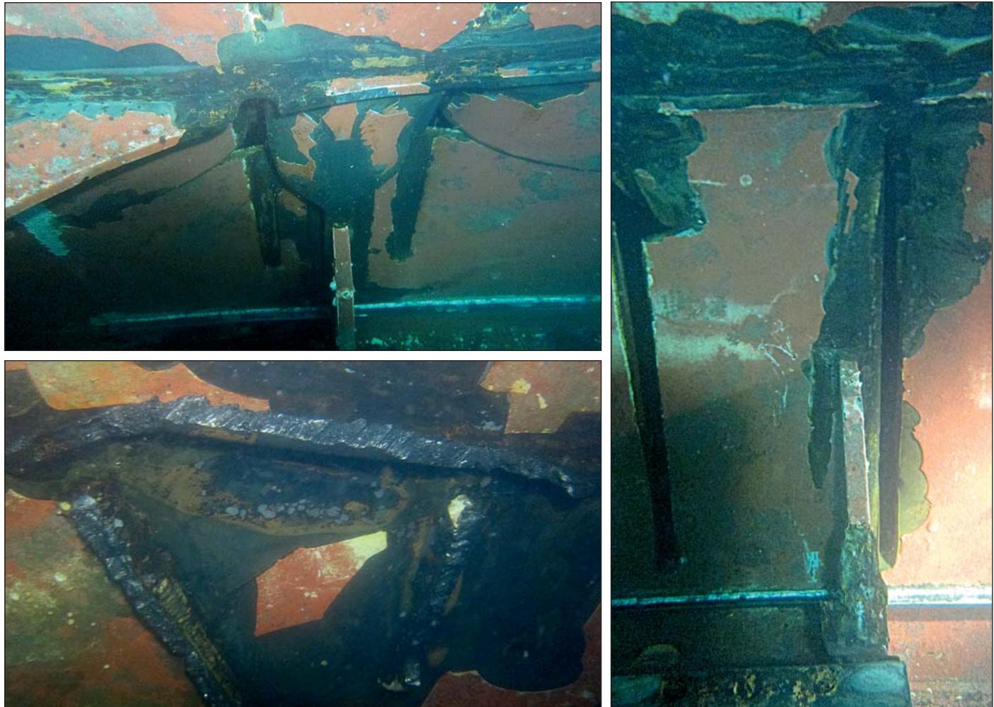
*Damage to the moonpool hull of drill ship, caused by loose transit flap.*
