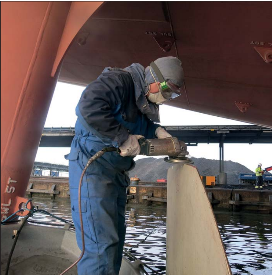
Grinding the edge of a modified propeller blade as per specifications.
