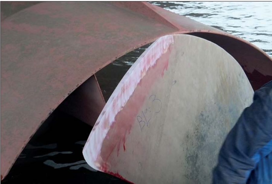
Testing one of the modified blades in Amsterdam for cracks.
