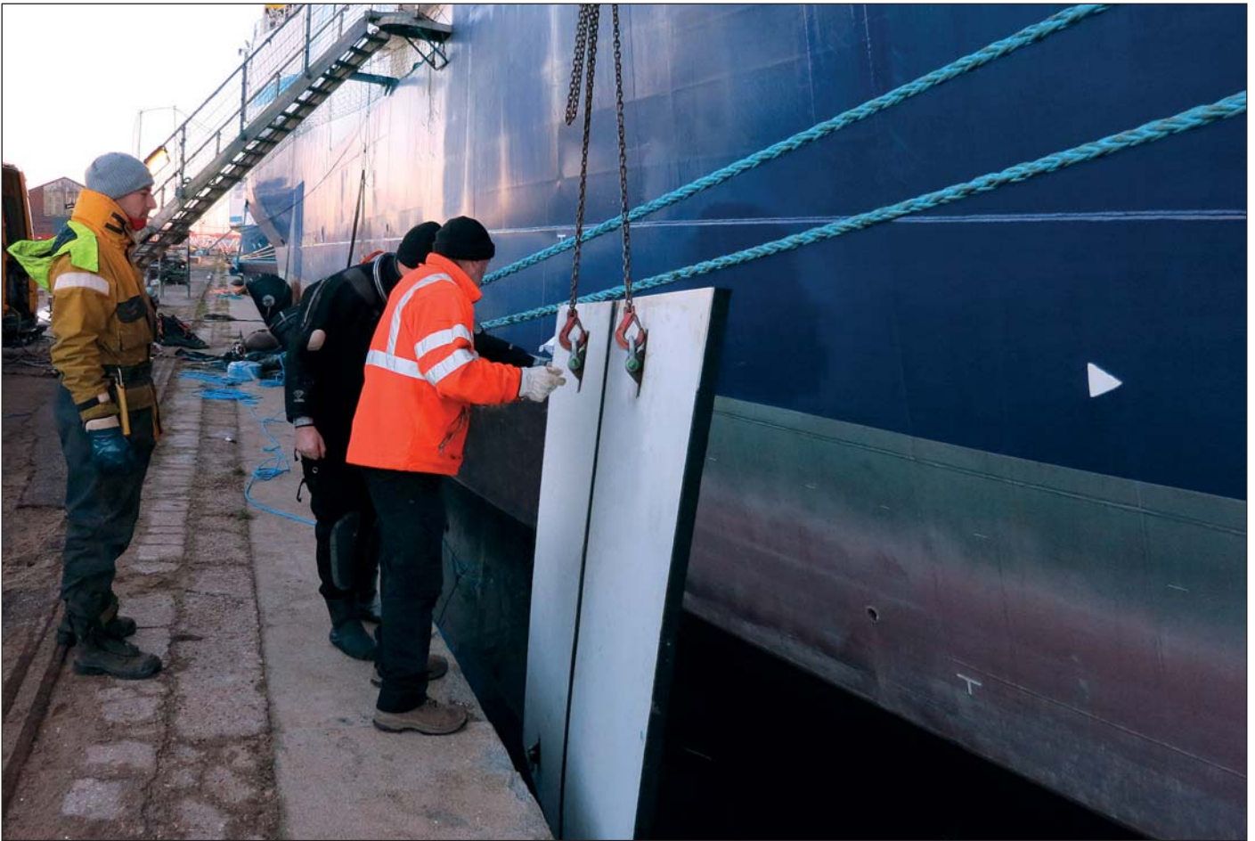
Lowering one of the blanks into the water.
