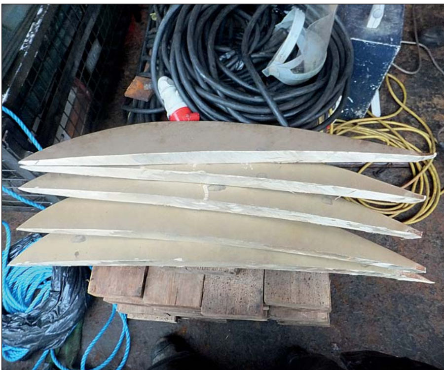
The propeller blades of two bulkers were modified to save fuel.
