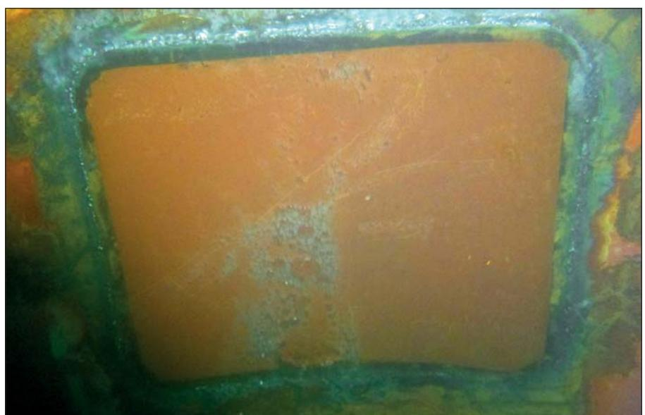
*One of the two doubler plates installed on the tanker.*
