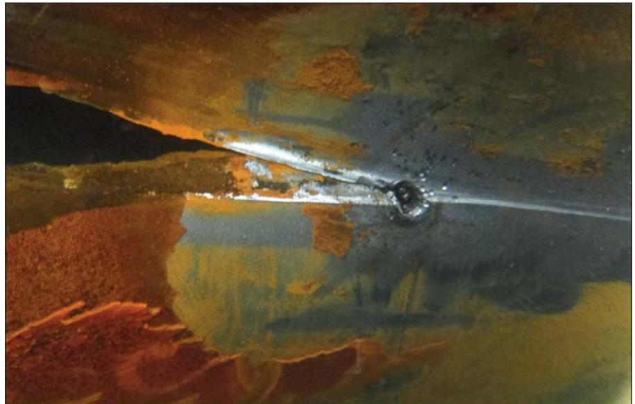
*Crack arrests were made on the extremities of all twelve cracks.*
