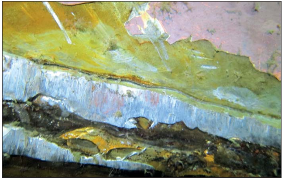
Damaged aft bulkhead area of drill ship.
