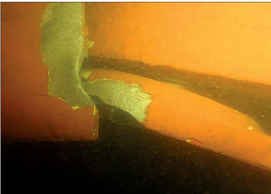
The edge of the rudder was cracked and bent.
