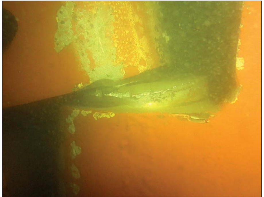
The rudder flap was almost completely detached from the rudder.
