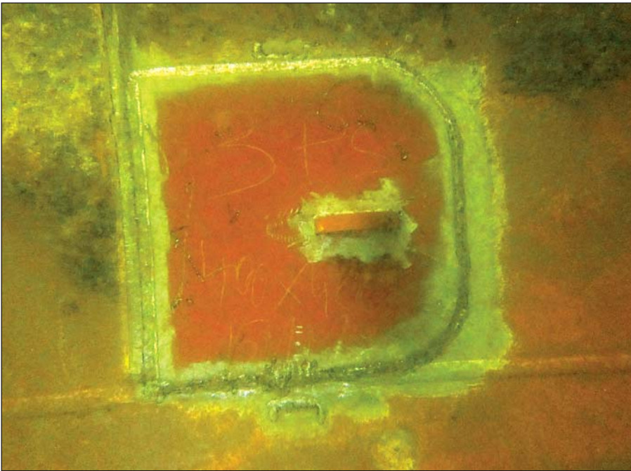
One of six doubler plates installed in Trinidad.
