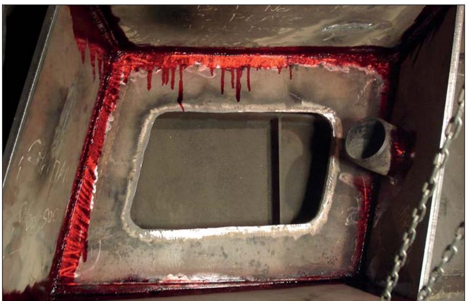
*Dye testing the weld seems of the newly installed box.*
