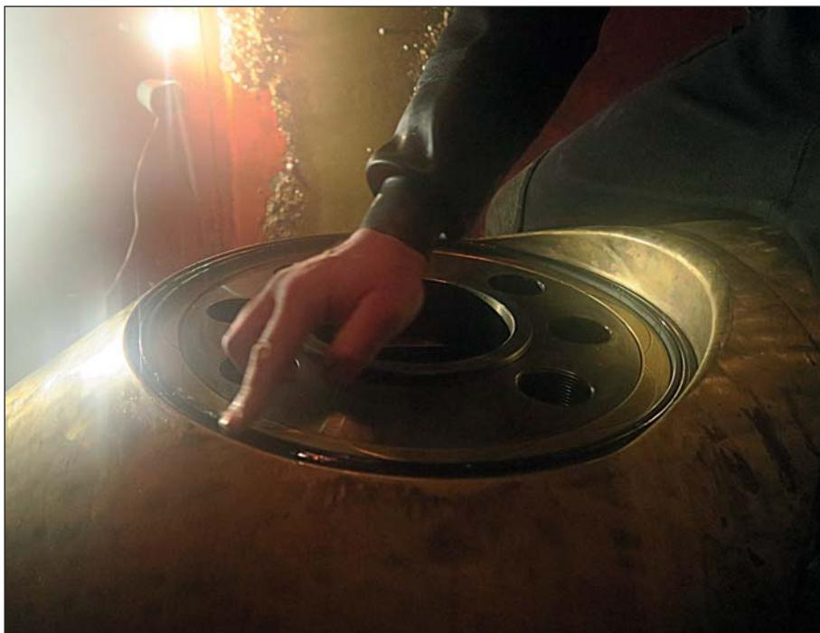
*Installing seal prior to reinstallation of thruster blade.*
