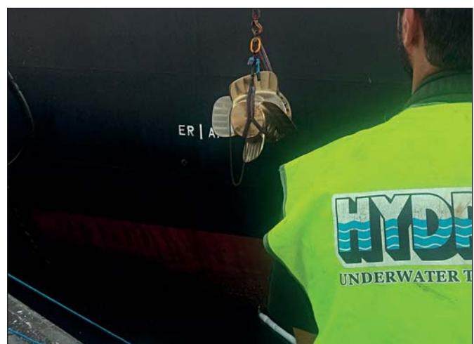
Hydrex technician lowering the propeller cone fin into the water.
