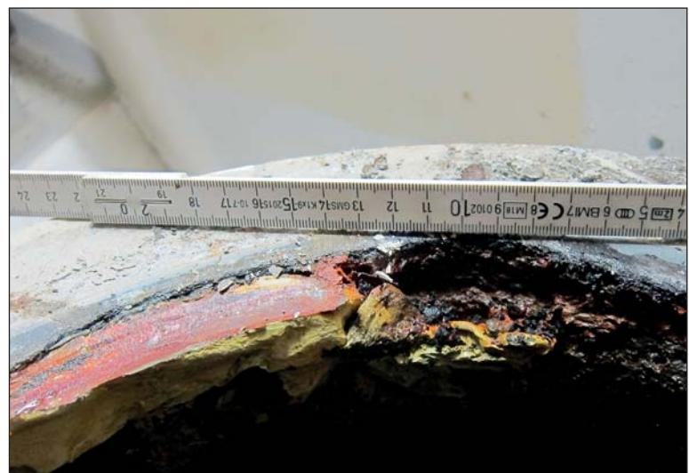
*The weld seam connecting the pipe to the flange was heavily corroded.*
