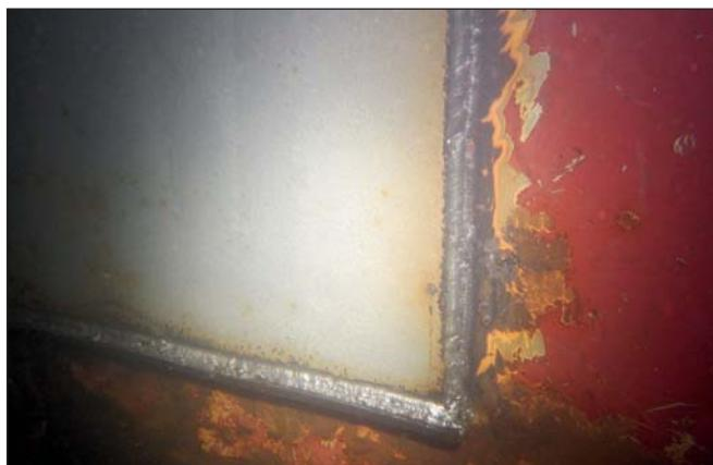
*Weld seams of doubler plate installed over damaged hull area.*
