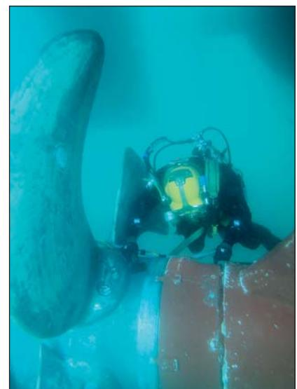
*Hydrex diver reinstalling the rope guard.*
