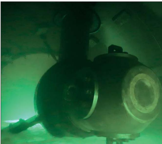
Overhauled unit in closed off thruster tunnel.
