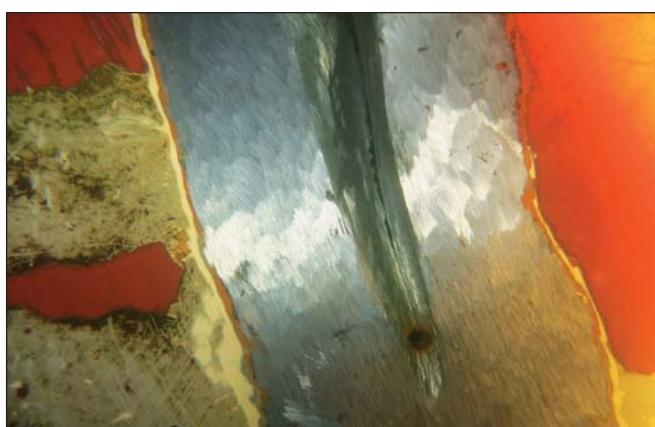
*Crack and the surrounding area cleaned and ground out.*
