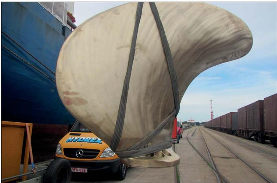
Propeller blade returning after the overhaul.
