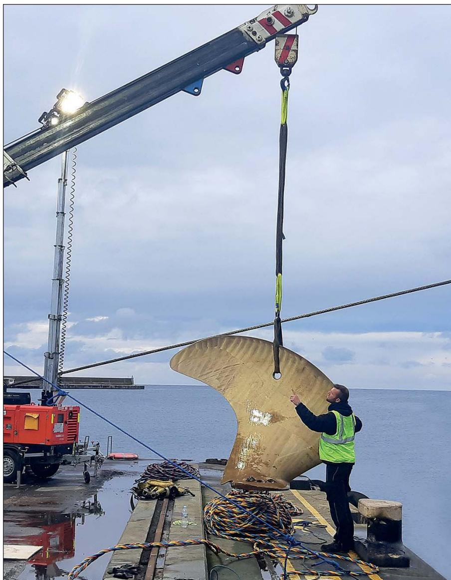
*Damaged propeller blade lifted on the dock.*
