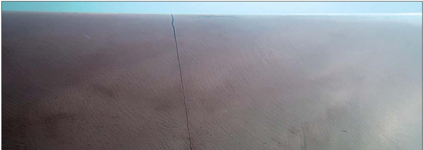
*The blade had suffered a very deep crack and needed to be replaced as per OEM recommendation.*
