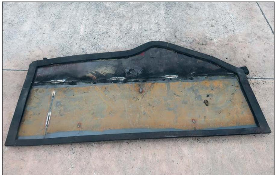
*A doubler plate was designed, fabricated and installed by our team on-site.*
