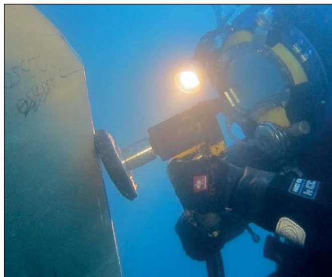
Hydrex diver grinding the edge of one of the cropped blades.
