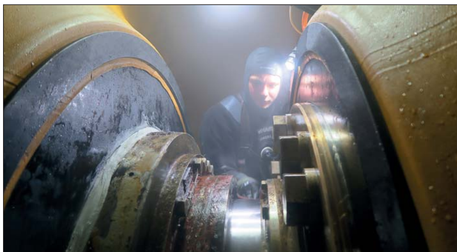
Diver inside our flexible mobdock during underwater stern tube seal repair in Rotterdam.
