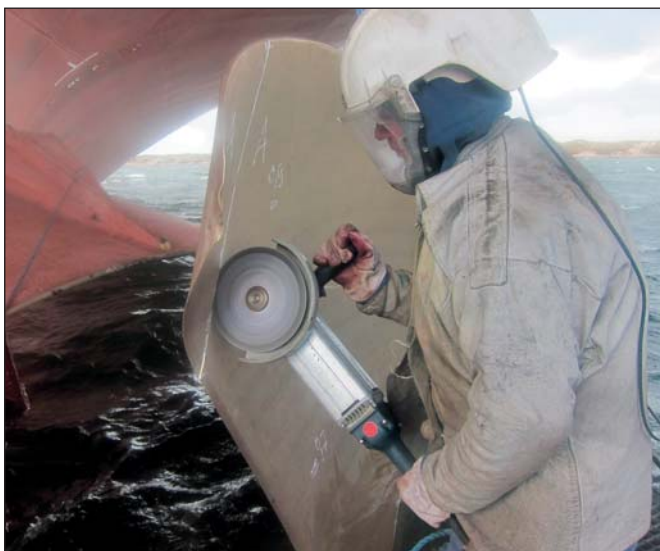
Hydrex technician cropping one of the blades in France.
