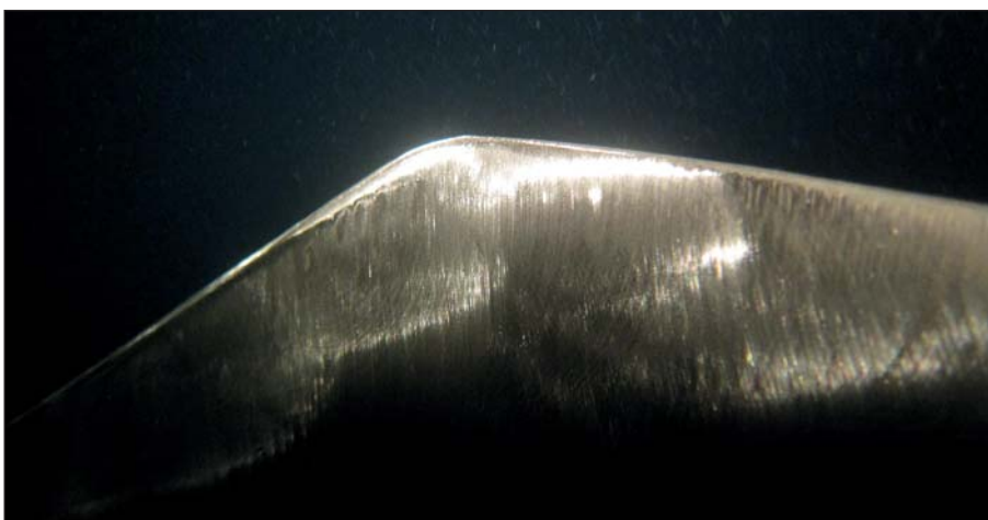
Polishing the cropped blades prevents performance loss.
