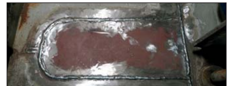
Permanent underwater insert repair on tanker in Amsterdam 10-11
