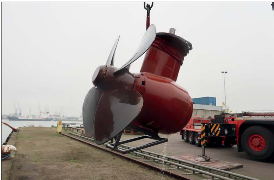
The thruster was removed without having to detach the blades.
