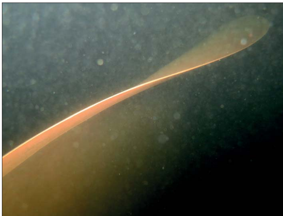
One of the bent blades of the bulker in Dunkirk.
