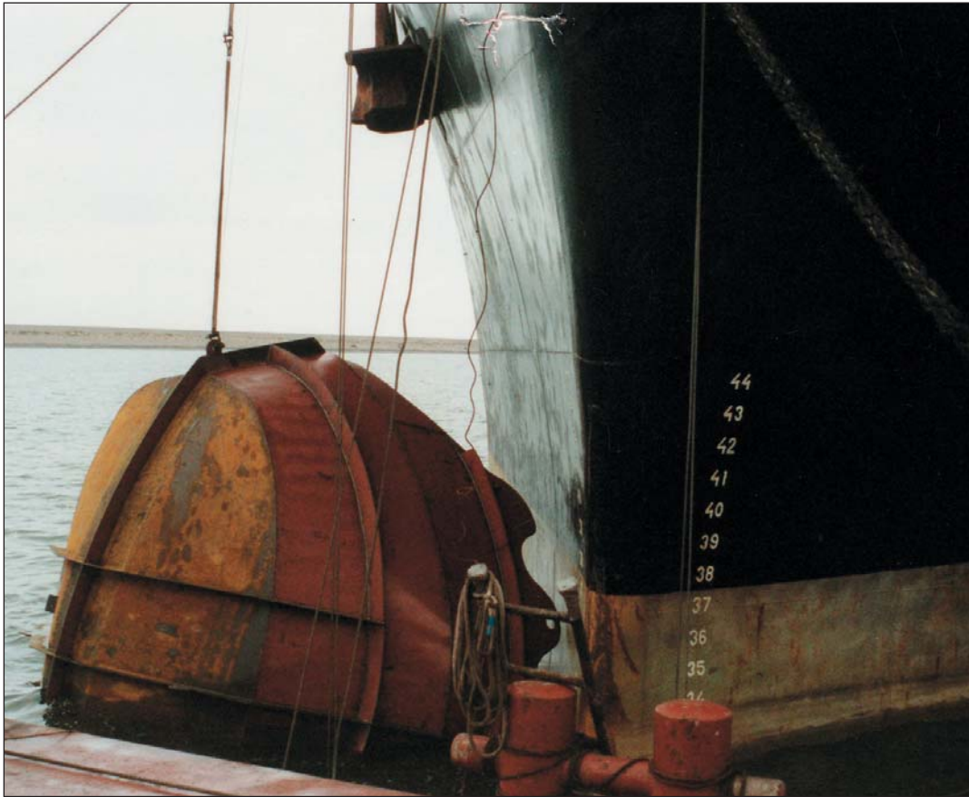
Hydrex took on the job of designing and constructing a shell to cover the damaged bulbous bow.
