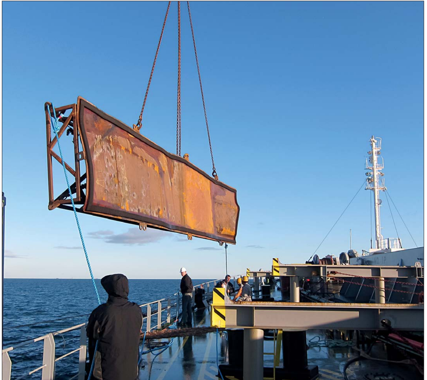
Preparing and lowering the doubler plate into the water so that it could be welded in place to repair the 8 x 1.8 m rip in the hull near the forepeak.
