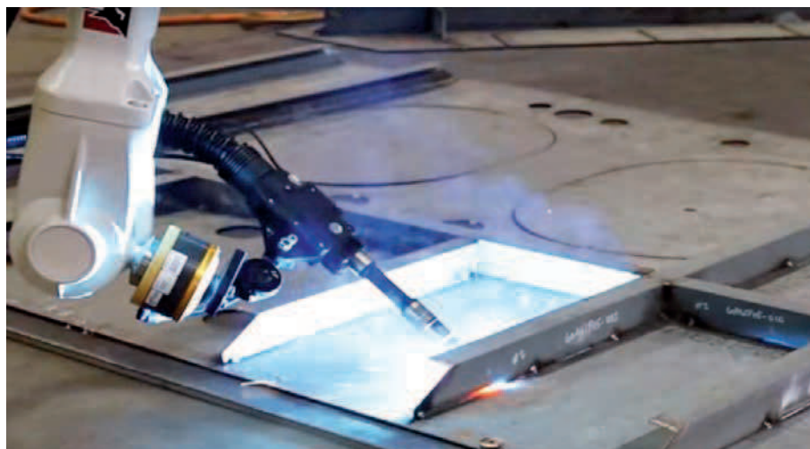
Figure 4: Computer-aided robotic welding (CAR-W) demonstrates the value of connection to underlying product model at Bollinger Shipyards
