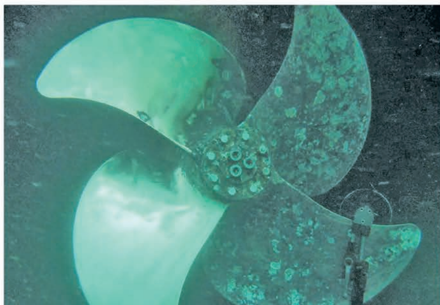
Figure 3: The company's buffing technique achieves a mirror-like shine, as shown on the left-hand blades of this propeller
