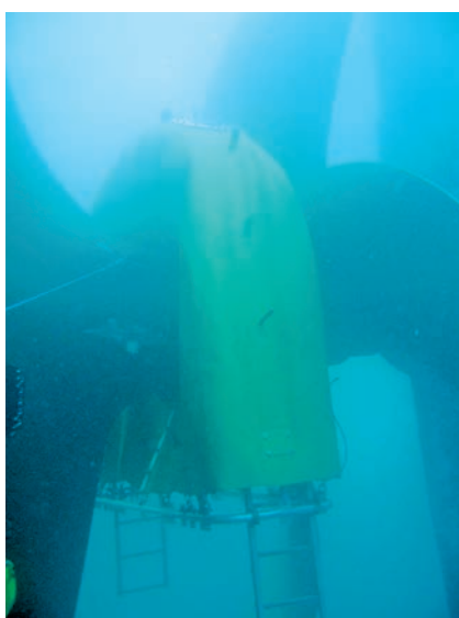
Figure 2: Hydrex's flexible mobdock is ideal for repairing stern tube seals
