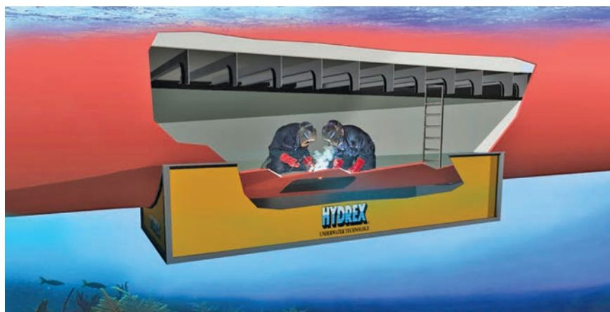
Figure 1: Large repairs are able to be carried out underwater thanks to Hydrex's tailored cofferdams
