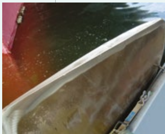
From top to cottom: The Hydrex team and equipment arriving on site; Cutting the opposite blade of the damaged propeller to keep the balance; The cropped and buffed blade
