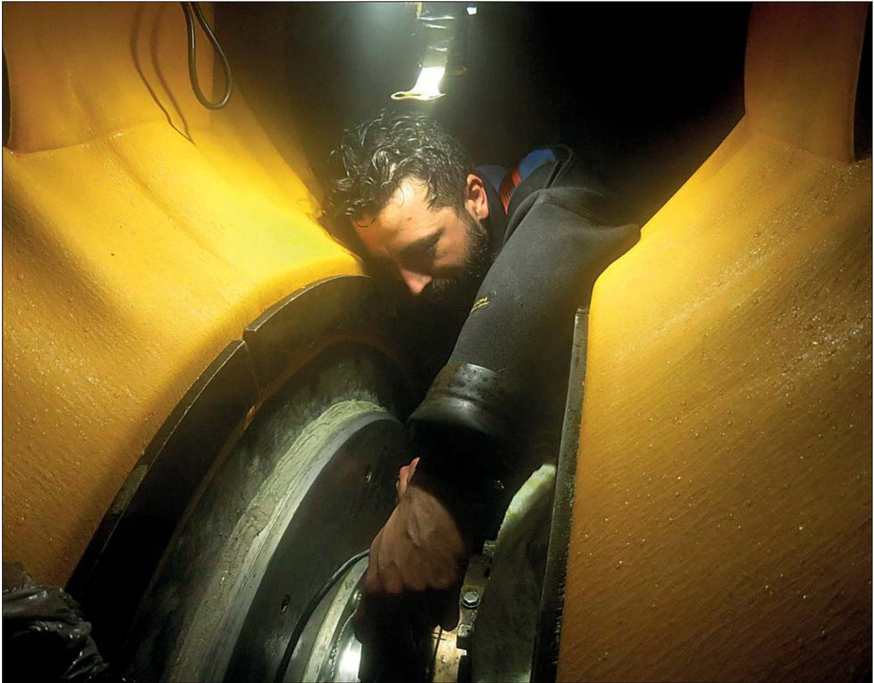
**U**sing our flexible mobdock method to create a dry underwater environment, we have carried out stern tube seal repairs and replacements underwater for some years now in cooperation with OEMs.
