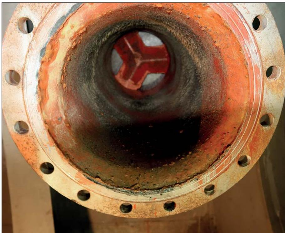
*Corroded scrubber pipe of bulker in Flushing.*
