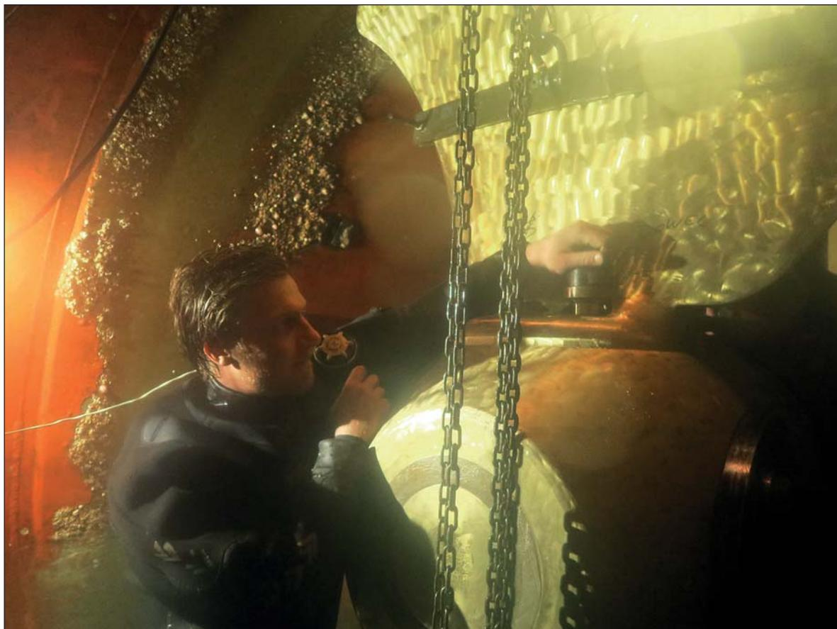
**T**he Hydrex lightweight flexible mobdocks are designed to be easily transported around the world and are used to close off the thruster tunnel on both sides, allowing divers to perform repairs and other operations in a dry environment around the bow thruster unit.
