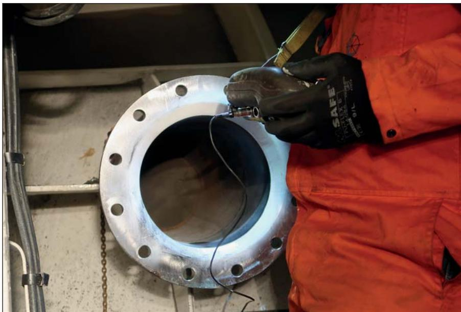
*Independent NDT testing of the welding work.*
