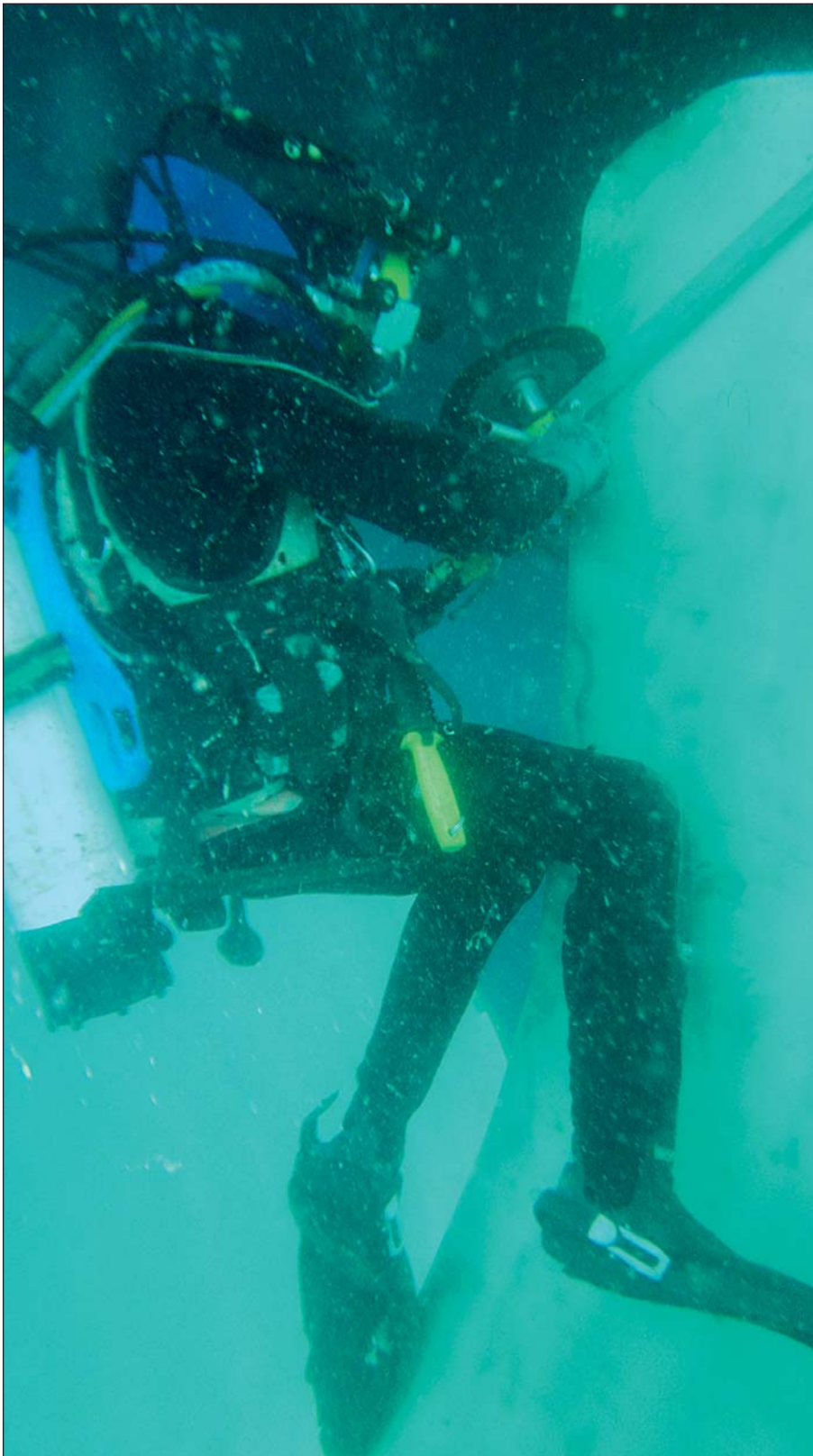
Blades can also be cropped underwater by our diver/technicians if needed.
