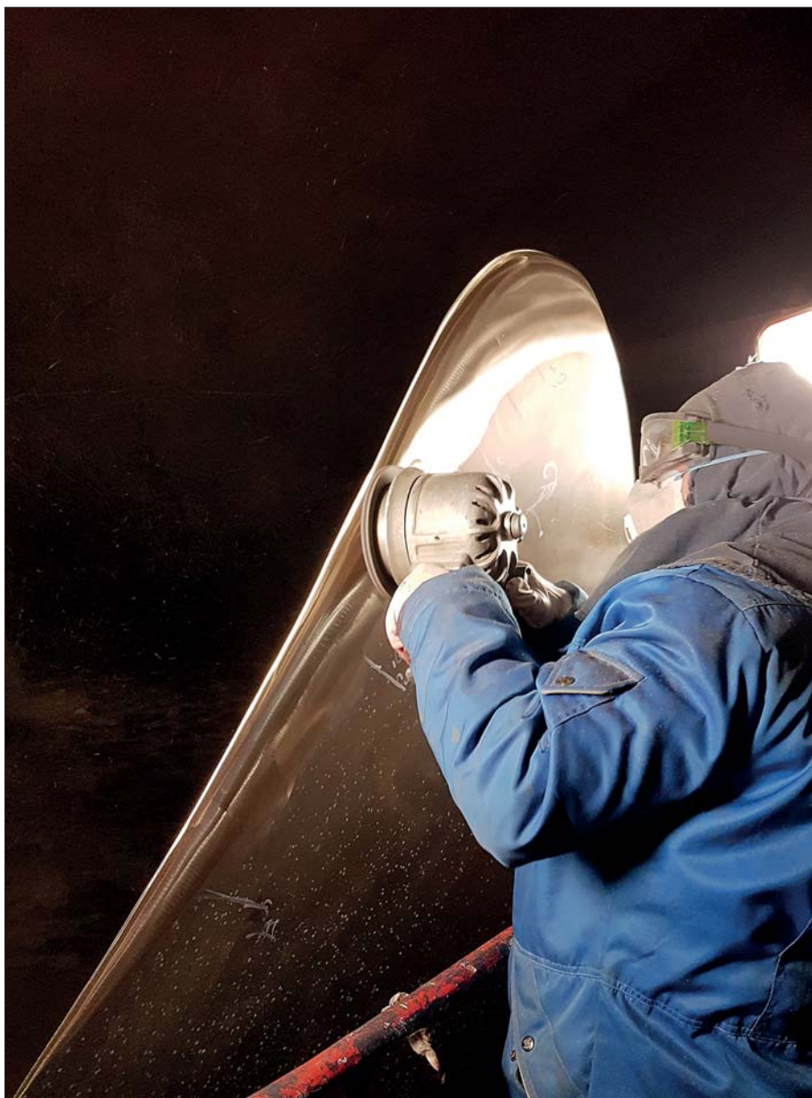
The edges of the affected blades are polished for maximum efficiency.
