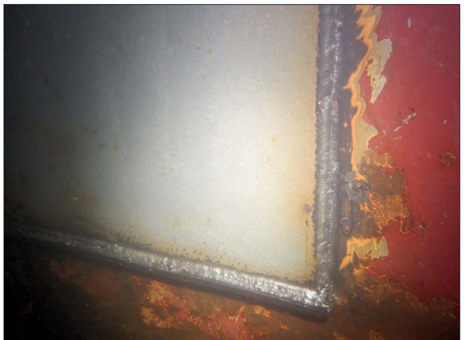
Weld seams of doubler plate installed over damaged hull area.
