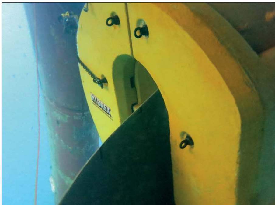
If possible, bent blades are restored with our cold straightening machine.
