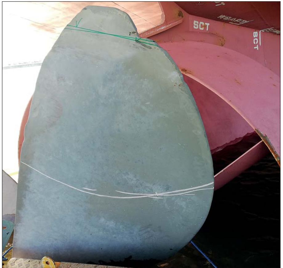
Trimmed propeller blade of bulker with damaged tip.
