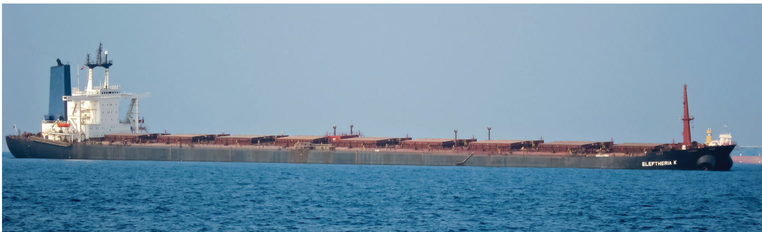
Fig. 2 — The ship at anchor near Fujairah, UAE. The ship has a severe list to starboard due to the leaks and flooding of the ballast tanks.
