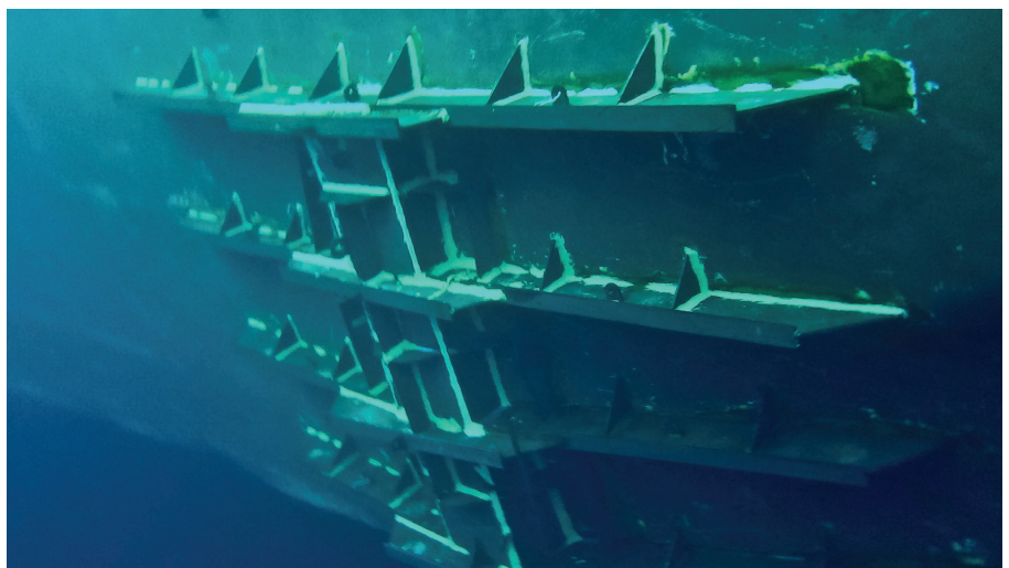
Fig. 16 — The finished repair. The welds were protected with epoxy to prevent corrosion.
