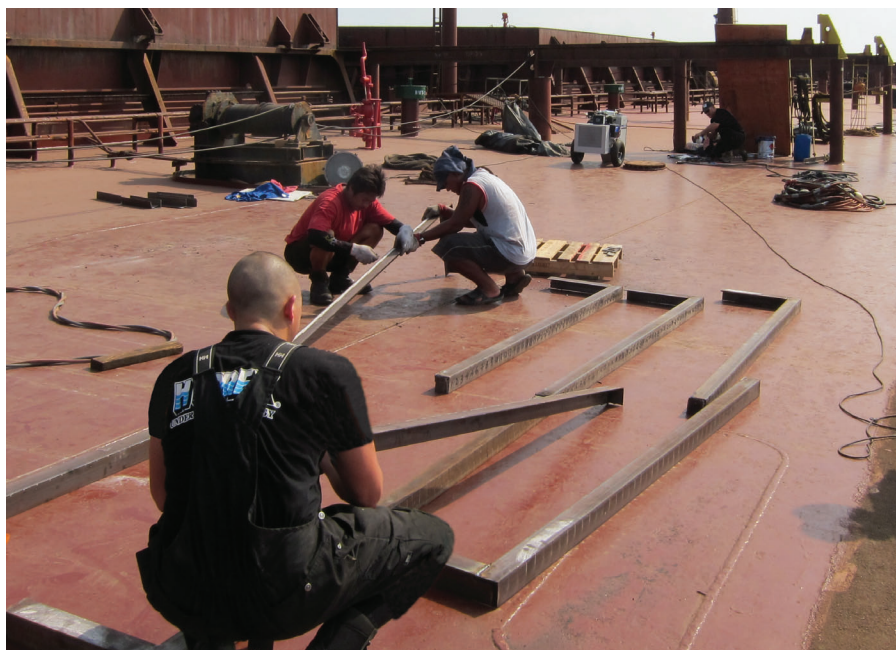
Fig. 9 — (Bottom left) The distorted shape of the hull was carefully measured in relation to the frame, with measurements taken every 5 cm, so the plates that would become the structure of the box could be accurately cut to fit.
