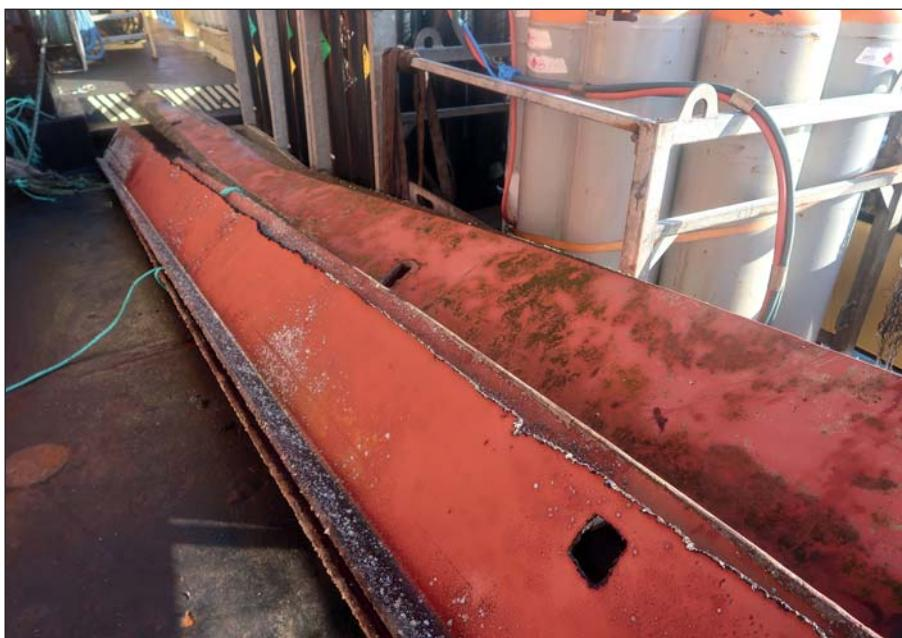
Removed section of bilge keel of oil tanker.
