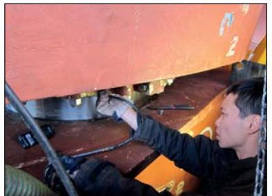
**H**ydrex has developed an entirely new method enabling permanent repairs of Rudders without drydocking the ship. Permanent repairs were hitherto not possible and ships had to drydock in case a major defect was found. The newly designed equipment is light-weight and can be mobilized very rapidly in our special flight containers. Therefore this new service is now available world-wide.
