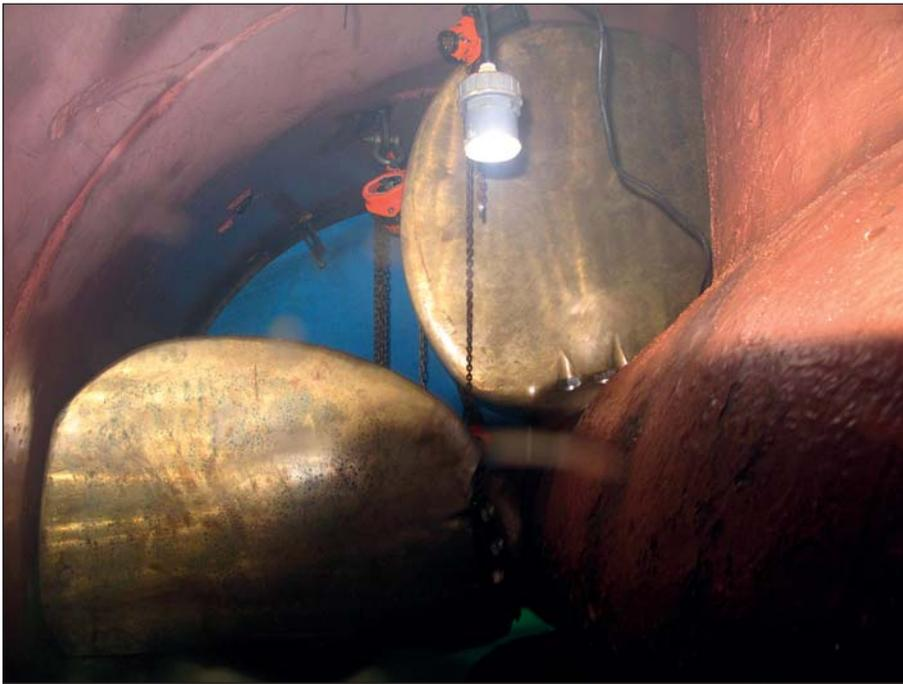
*Reinstalled bow thruster unit inside closed off thruster tunnel.*
