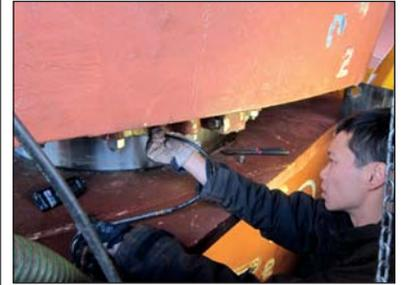
**H**ydrex has developed an entirely new method enabling permanent repairs of rudders without drydocking the ship. Permanent repairs were hitherto not possible and ships had to drydock in case a major defect was found. The newly designed equipment is light-weight and can be mobilized very rapidly in our special flight containers. Therefore this new service is now available world-wide.
