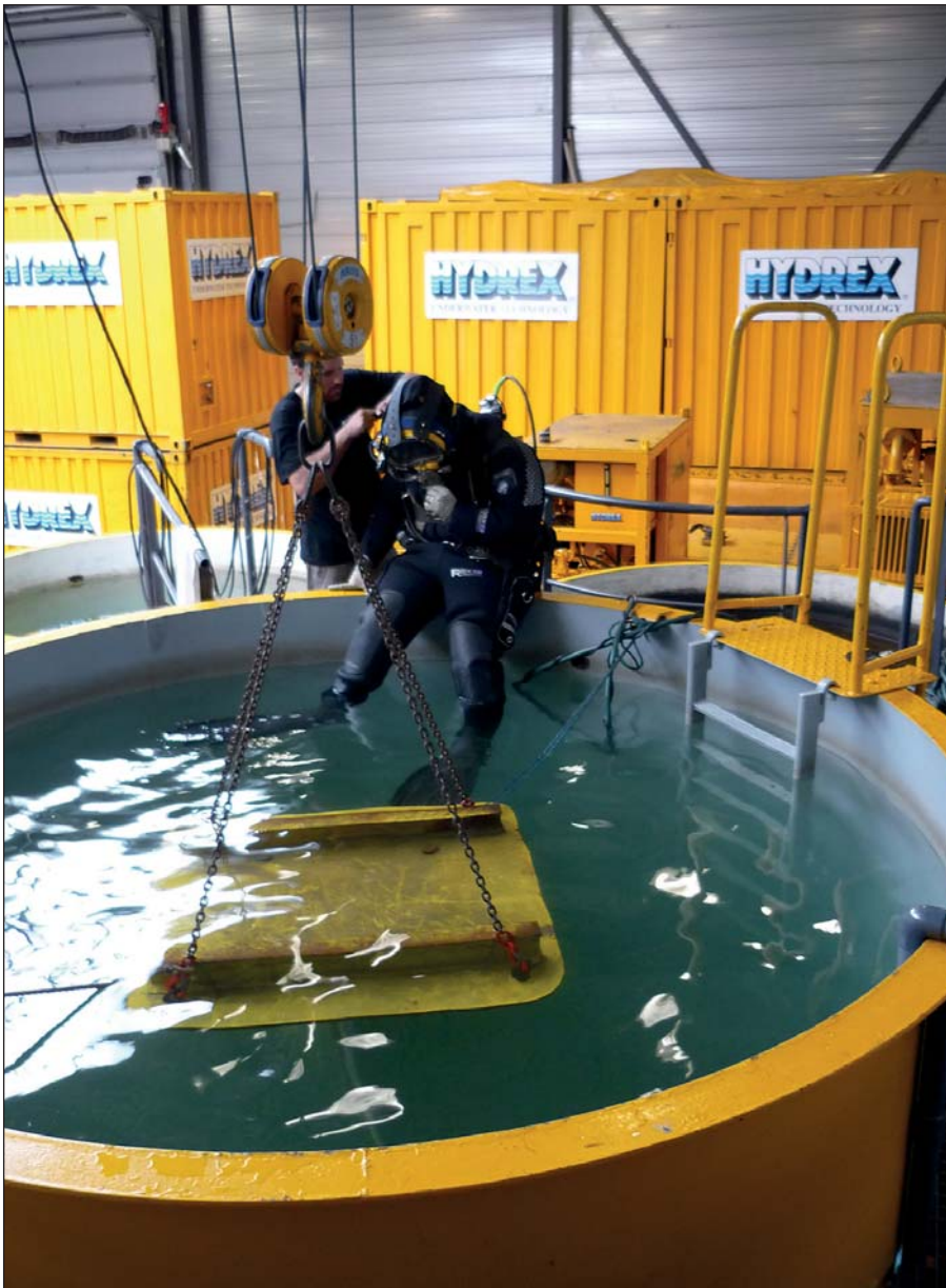
Our training facilities include three dive training tanks to practice underwater welding and other repair work.
