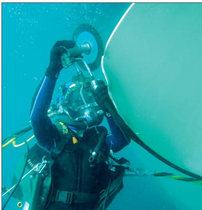
Any type of propeller modification can also be carried out underwater.
