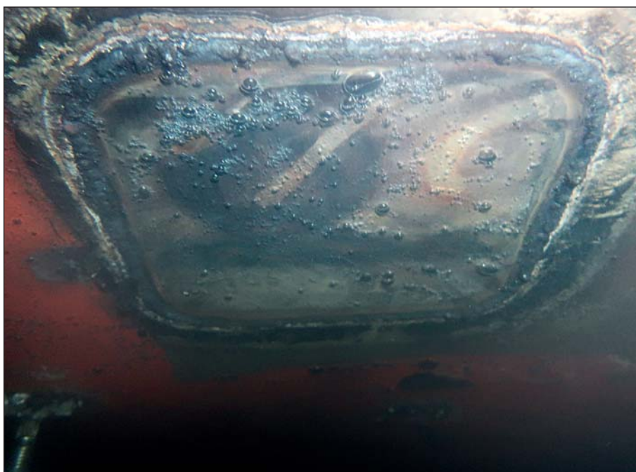
New insert plate seen from the waterside.
