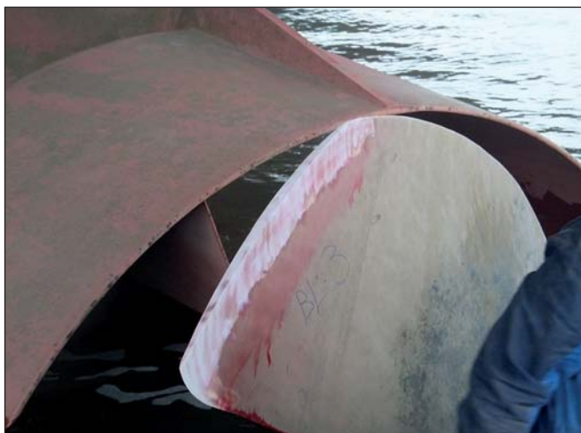
Testing one of the modified blades in Amsterdam for cracks.
