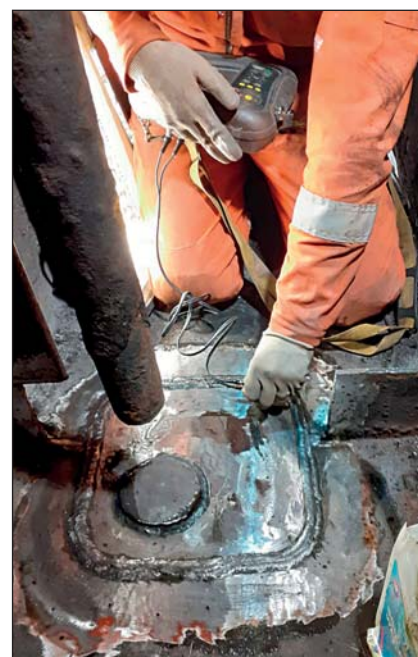
An independent inspector carried out ultrasonic testing.
