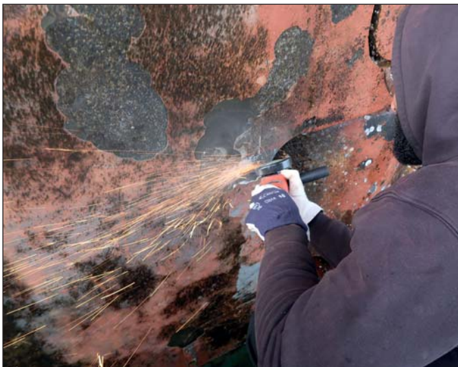
Hydrex technician grinding out the crack in Le Havre on the trimmed vessel.
