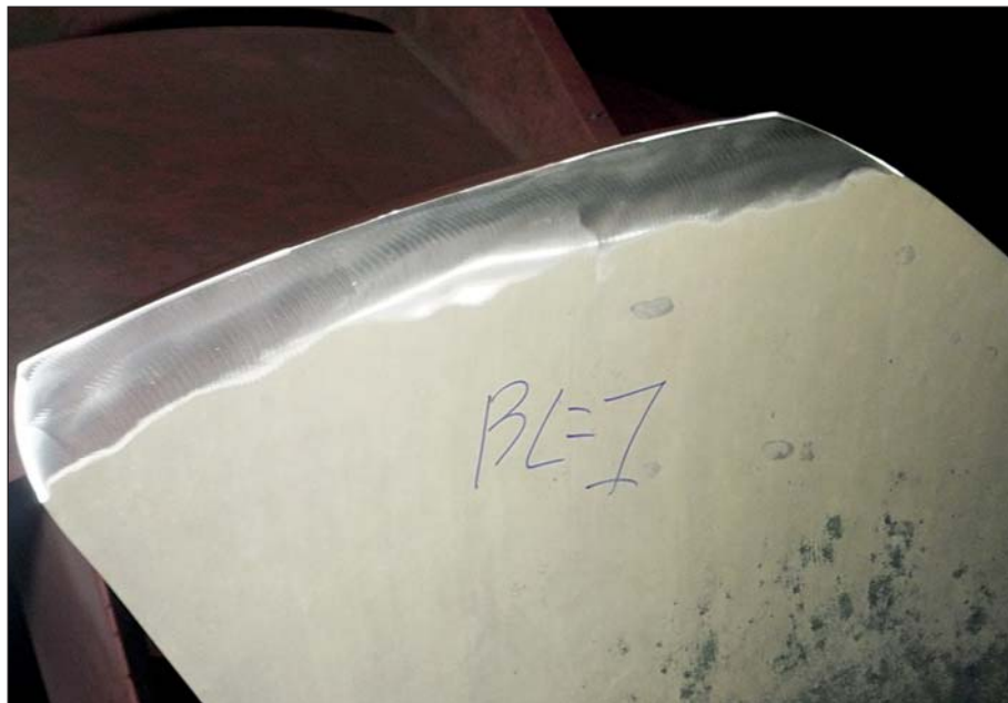
Modified propeller blade of bulker in Rotterdam.
