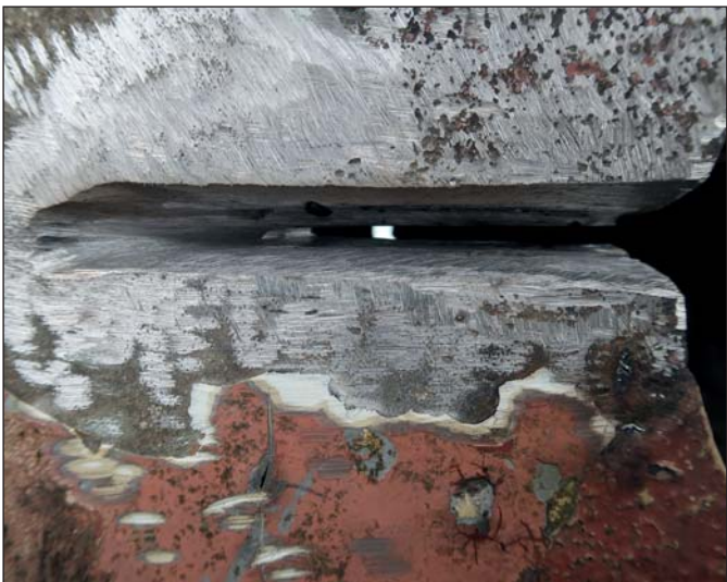
Ground out crack, ready to be filled.
