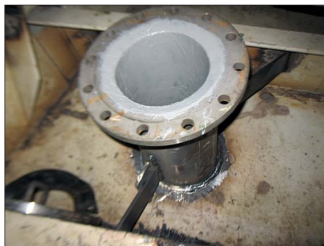
New overboard scrubber pipe with Ecospeed protection on the inside.
