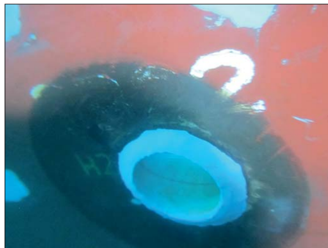
Outlet of one of six new scrubber pipes on second container vessel.
