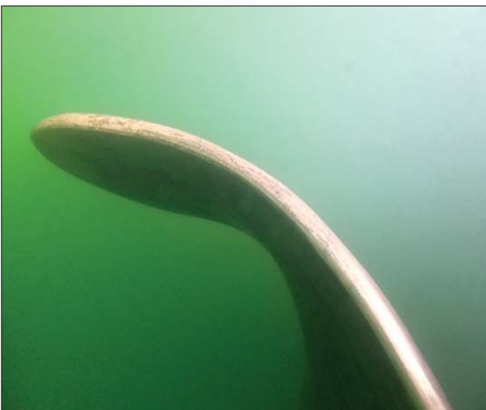
Bent propeller blade on bulker in Rotterdam.
