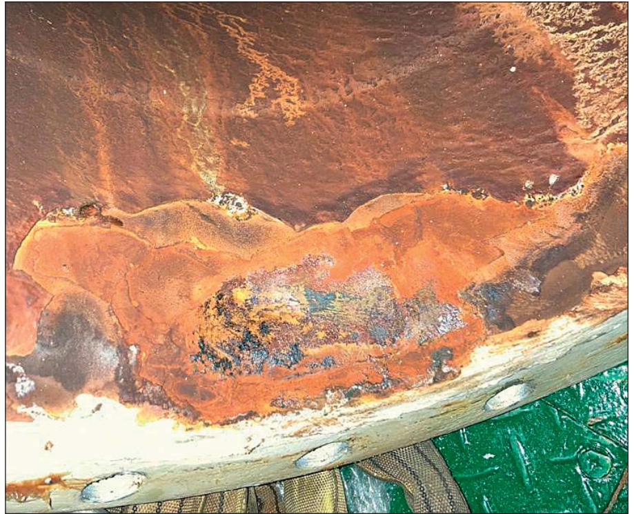
Corroded scrubber pipe of oil tanker in Le Havre.
