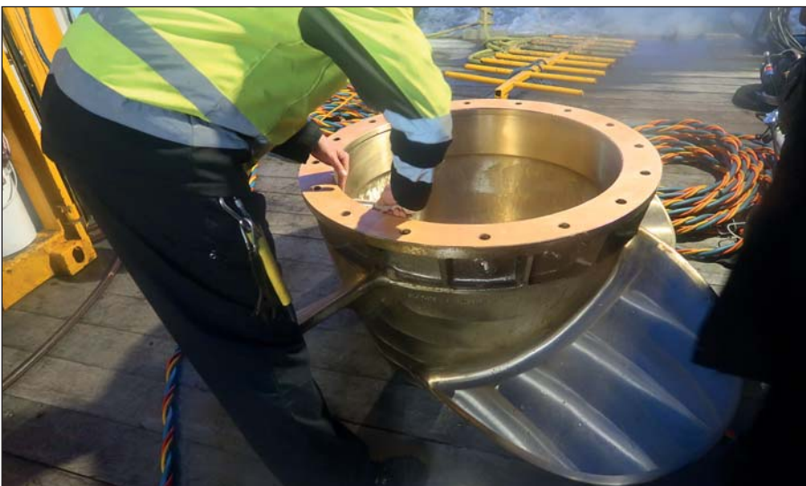
Preparing the propeller cone fin for installation.
