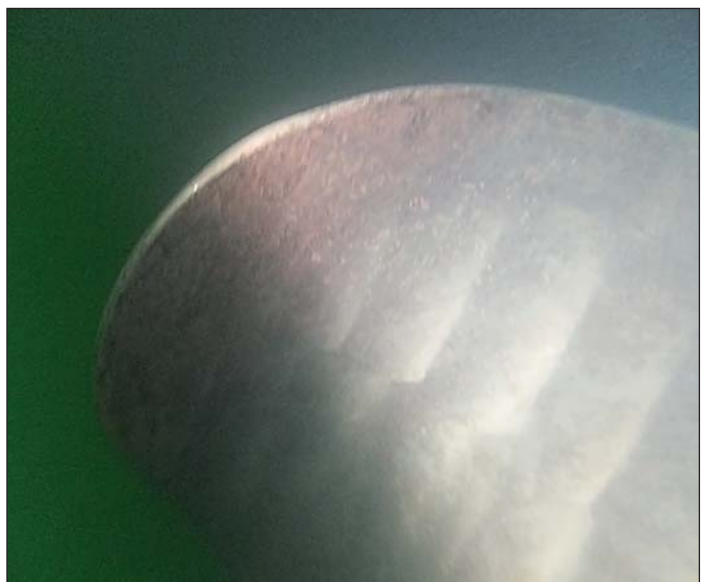
Propeller blade after straightening.
