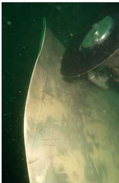
Cropping one of the blades of bulker in France.
