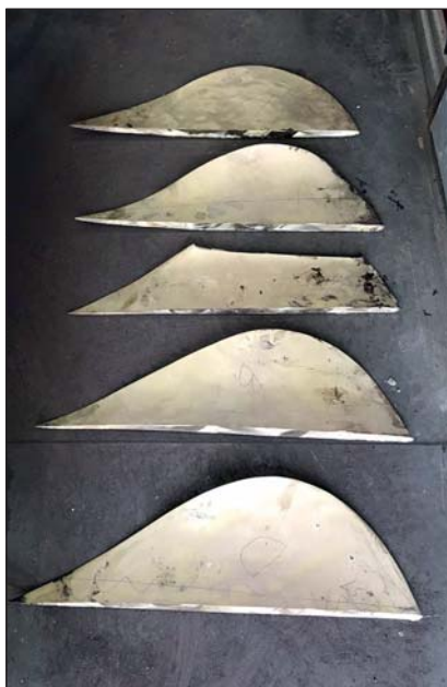
Cropped tips of the five propeller blades in France.
