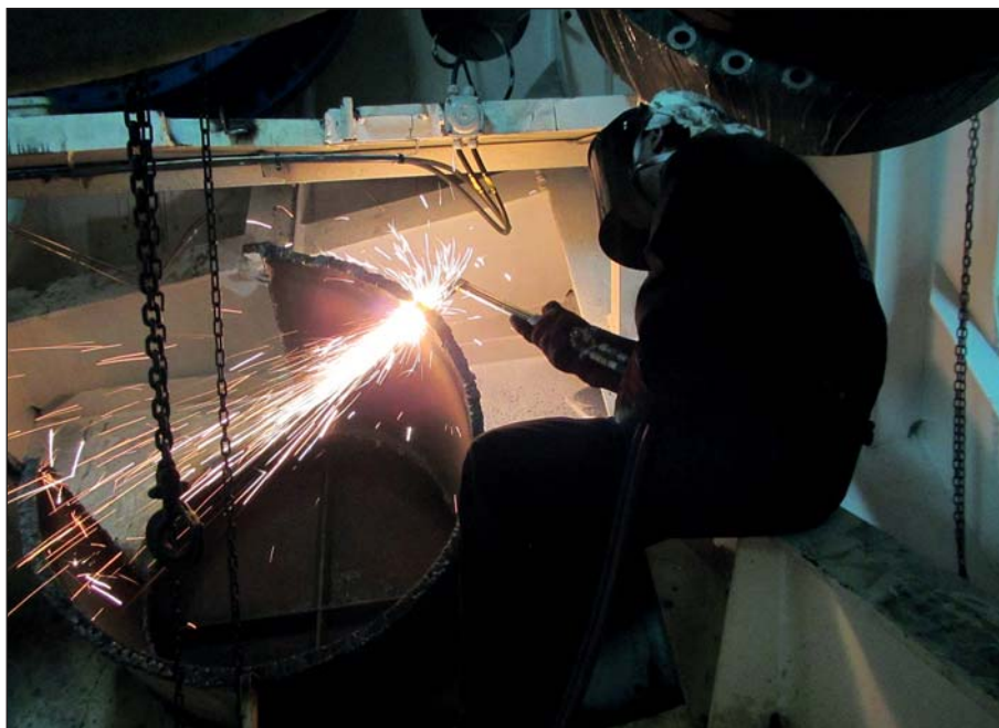
Cutting away the damaged pipe on container vessel.
