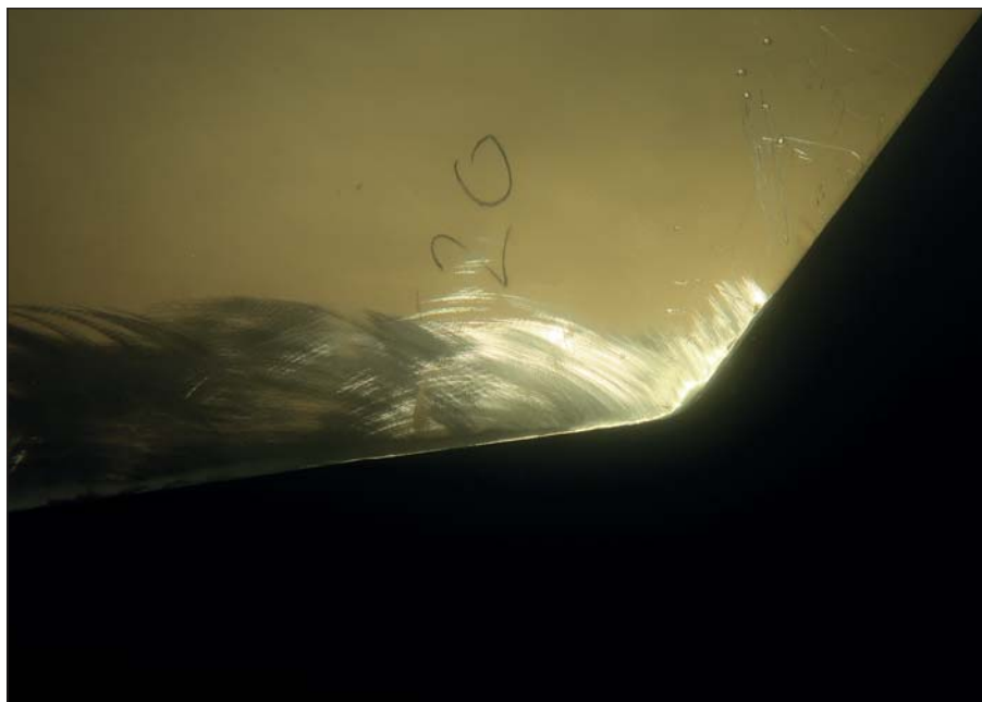
Propeller blade of bulker in Germany after cropping and smoothing.
