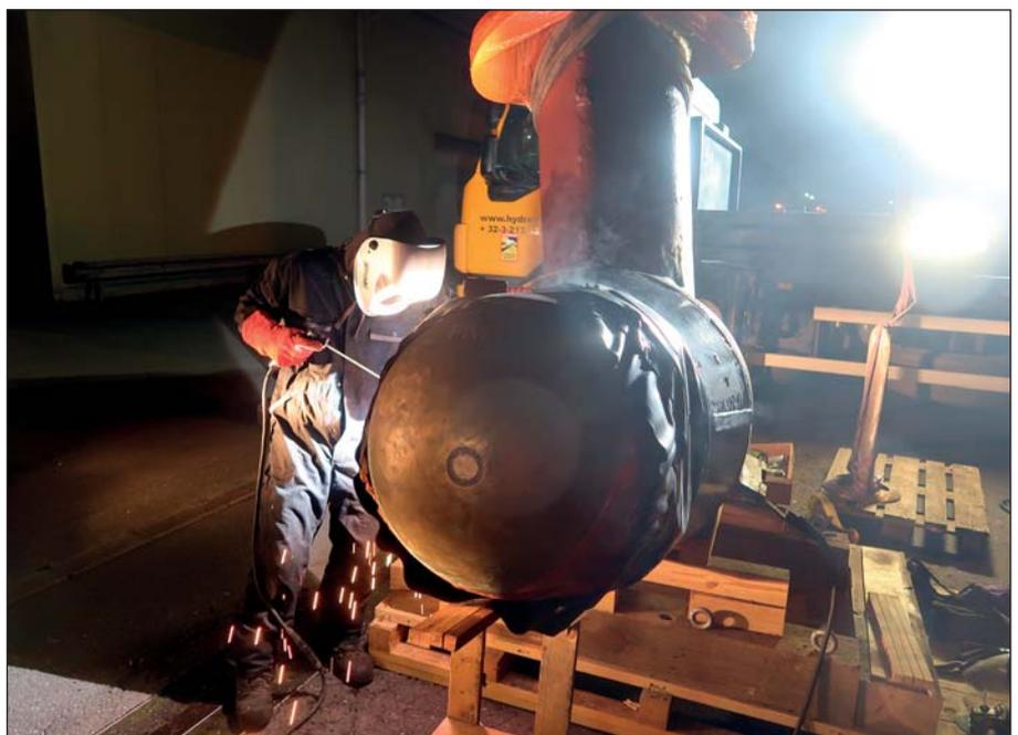
*Preparing the bow thruster in Zeebrugge for reinstallation.*
