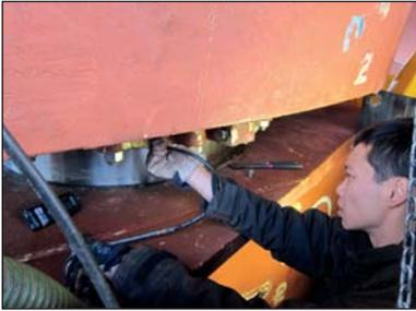
**H**ydrex has developed an entirely new method enabling permanent repairs of rudders without drydocking the ship. Permanent repairs were hitherto not possible and ships had to drydock in case a major defect was found. The newly designed equipment is light-weight and can be mobilized very rapidly in our special flight containers.
