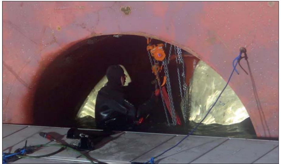
*Hydrex diver securing the bow thruster.*
