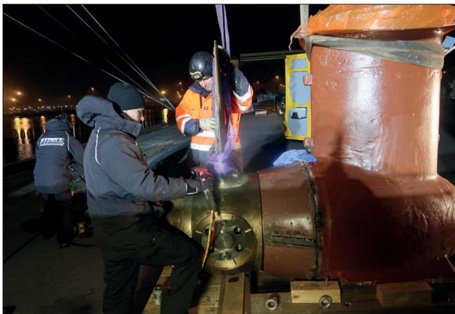
*Reinstalling the bow thruster blades.*
