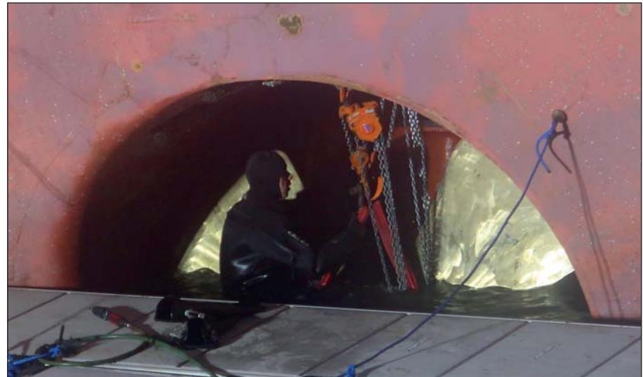
*Hydrex diver securing the bow thruster.*
