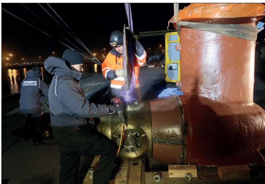
Reinstalling the bow thruster blades.
