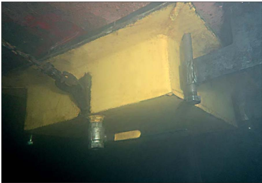
*Cofferdam installed on the hull of tanker in Rotterdam.*
