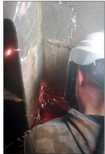
*Grinding out crack on ro-ro ship.*
