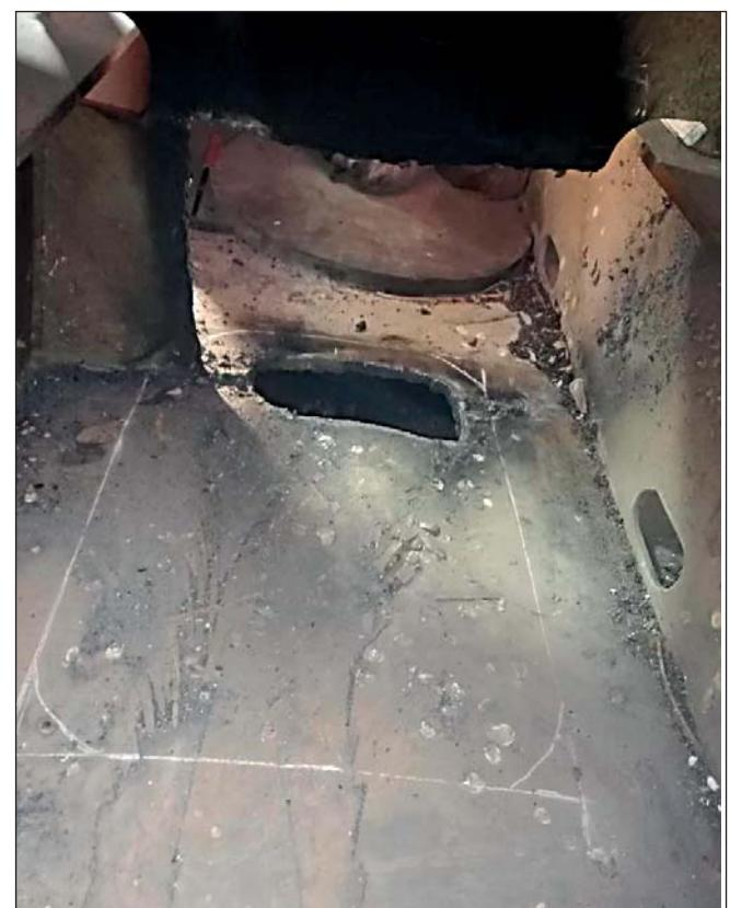
*Damaged shell plating on container ship in Rotterdam.*
