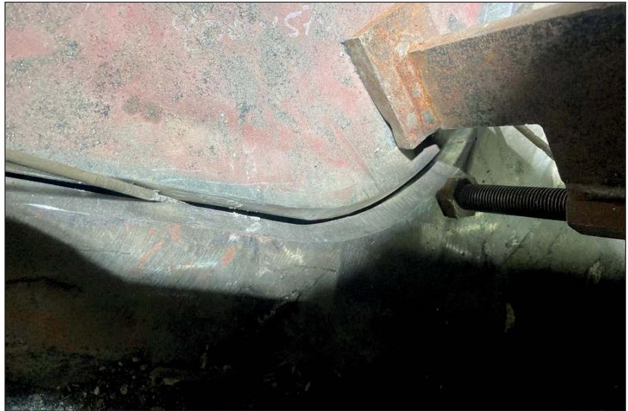
New insert secured and ready for welding.
