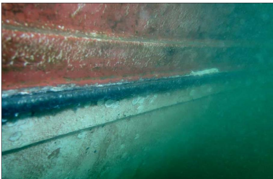
One of the damaged bilge keel sections after cropping.
