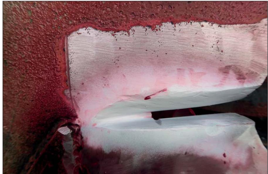
*Ground out crack ready for rewelding.*
