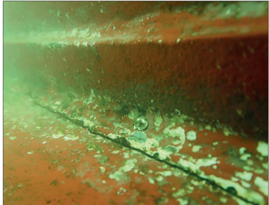
*The bilge keels on both sides of the tanker had suffered several large cracks.*
