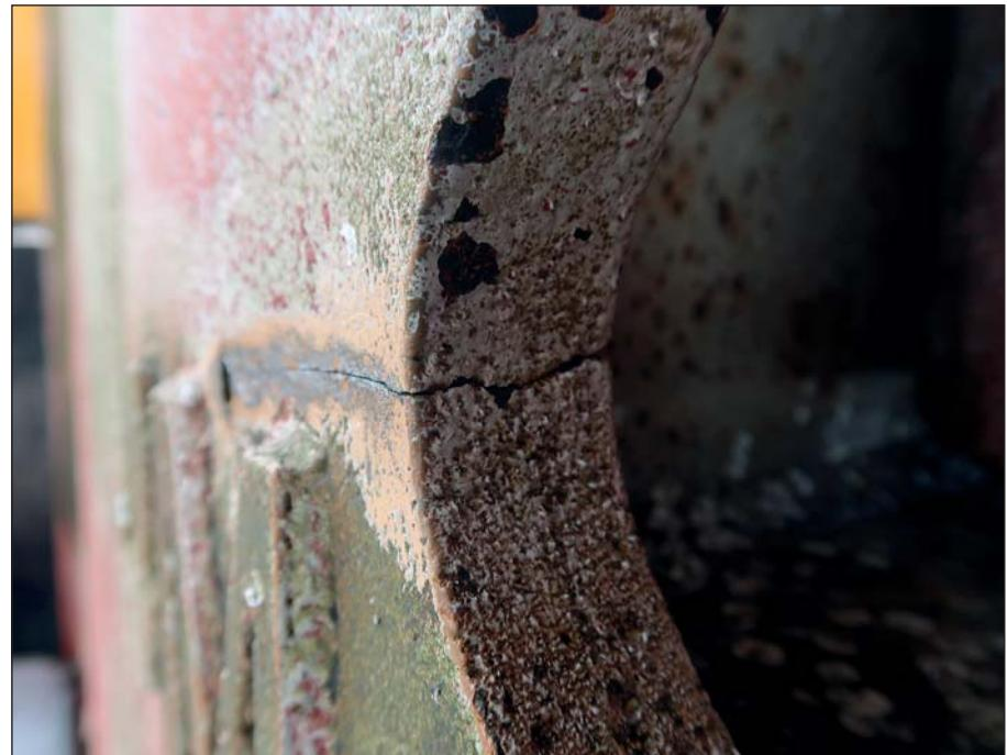
*One of the cracks in the pintle corners of the rudder.*
