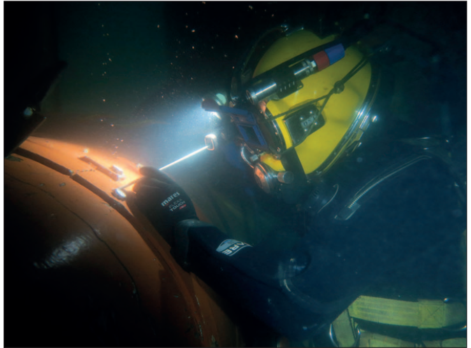
One of our divers working on the rope guard of car carrier in Tasmania.
