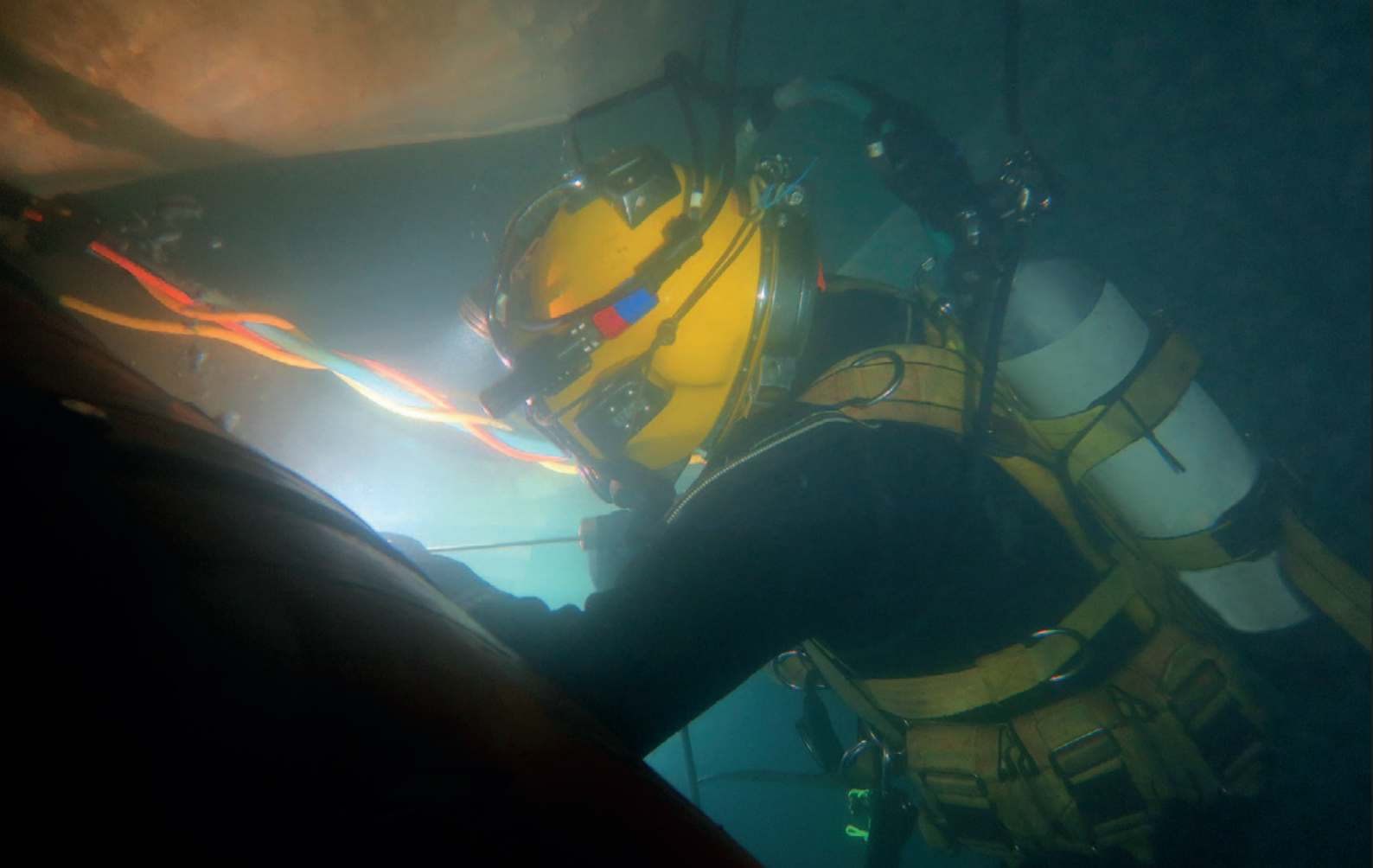
Hydrex diver reinstalling the rope guard.
