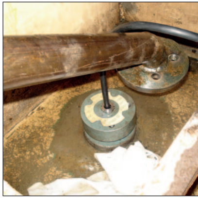
Any type of transducer can be installed or replaced afloat.
