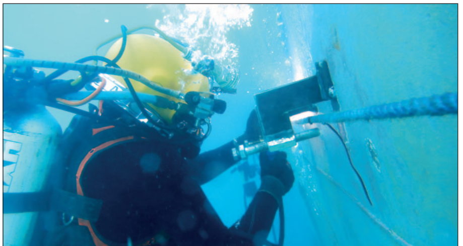
Preparing the hull for installation of the flexible mobdocks.
