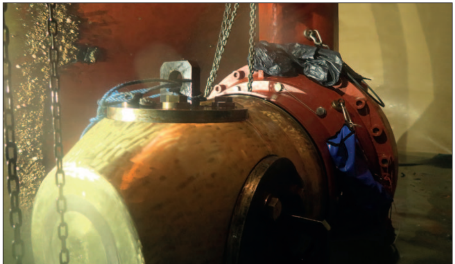
Thruster unit in closed off tunnel.
