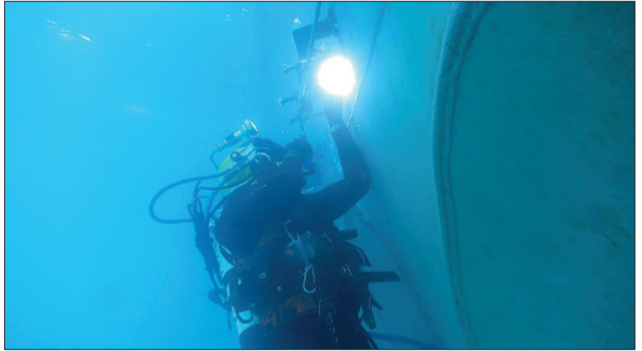
Diver performing welding work on the hull of offshore supply vessel in Australia.
