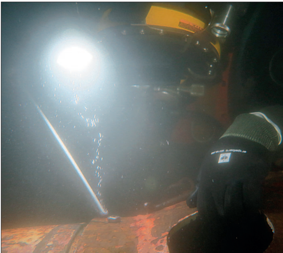
Hydrex diver securing the bolts on a rope guard.
