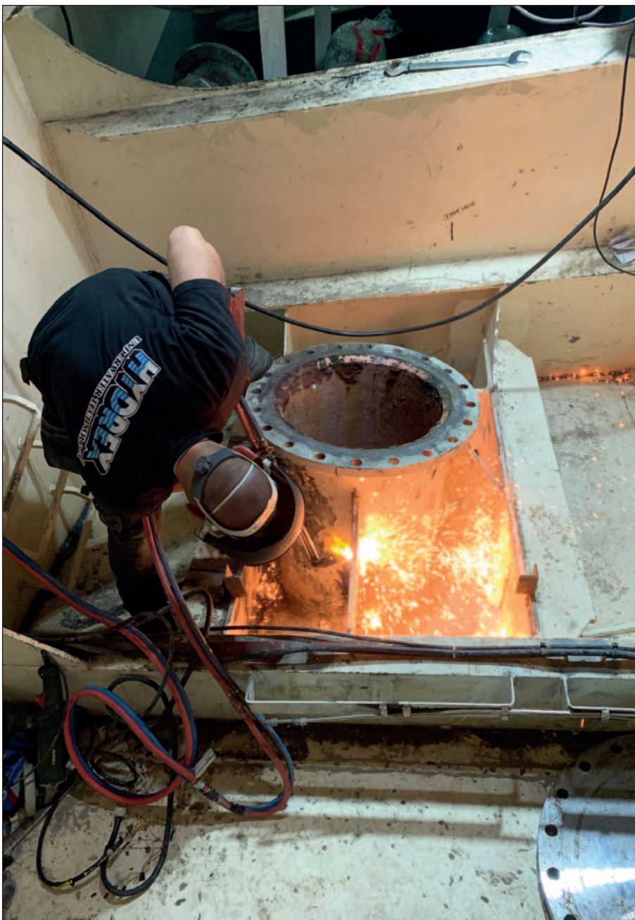
Removing the old scrubber pipe.
