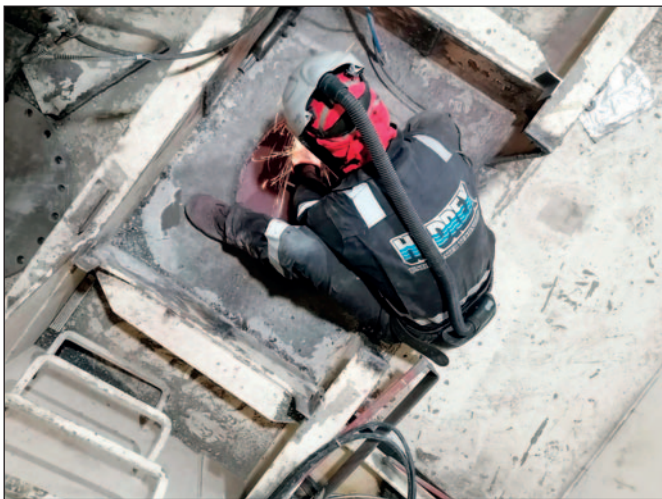
Preparing the edge of the shell plating for a new scrubber pipe.
