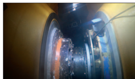
Double stern tube seal repair on pipe laying vessel in Rotterdam
